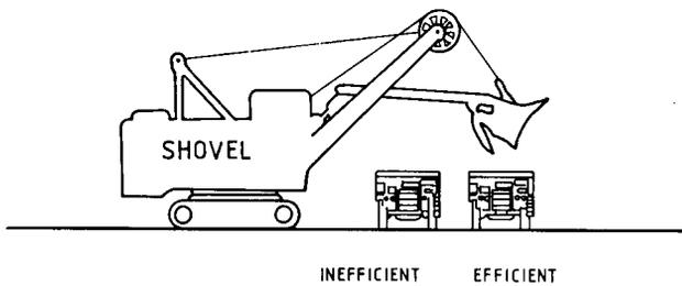
Fig. 5—Truck-loading technique
