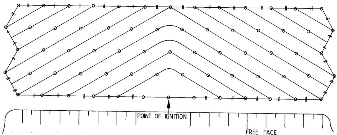
Fig. 4—Present drilling and firing patterns
