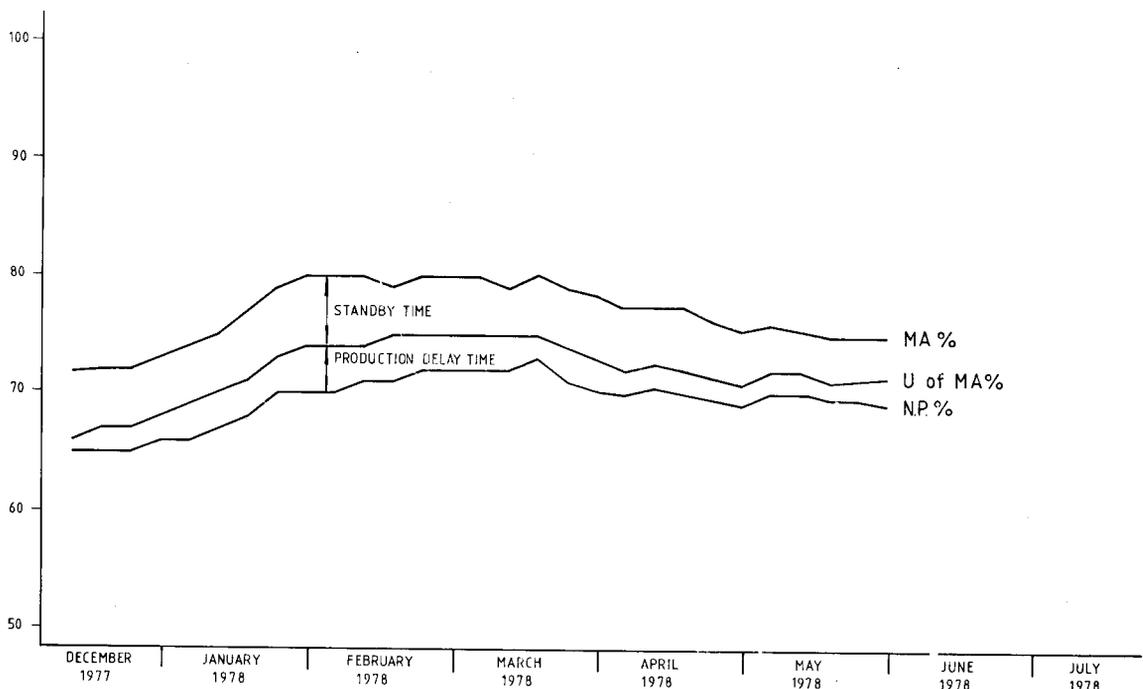
Fig. 10—Exponentially weighted moving averages of the availabilities of the 150t Wabco trucks
