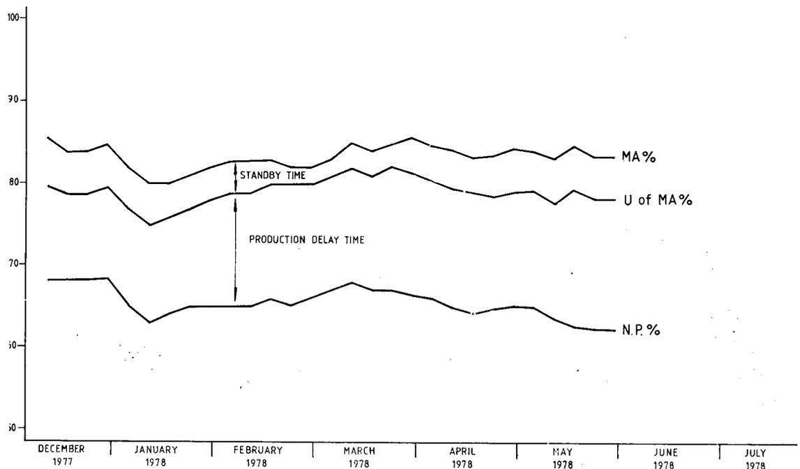
Fig. 9—Exponentially weighted moving averages of the availabilities of the P&H 2300 15.3 m shovels
