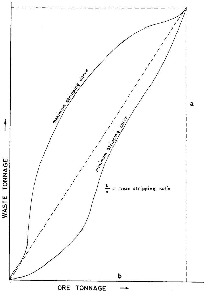
Fig. 2—Example of the stripping curves obtained from the MPS at a marginal volumetric stripping ratio of 4,3 to 1
