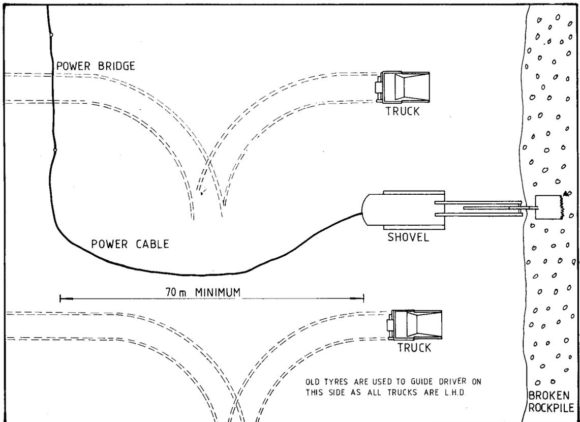
Fig. 6—Double-sided loading technique (It should be noted that no 'spotters' are used; instead, the trucks are reversed so that the driver's cabin is on the inside radius and the driver can see one of the rear wheels)
