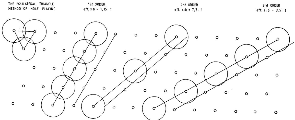
Fig. 3—The three ways in which equilateral-triangular hole placings can be tied in to achieve different effective s:b ratios
