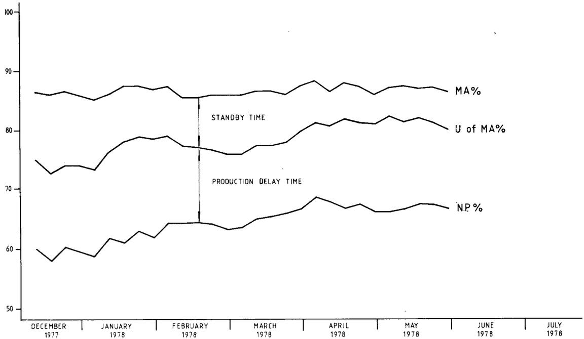
Fig. 8—Exponentially weighted moving averages of the availabilities of the 310 mm Gardner Denver rotary drills
