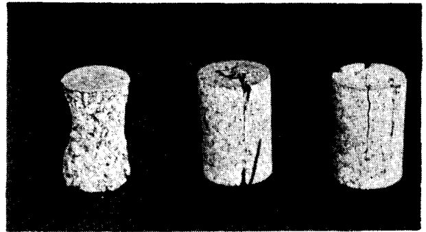
Fig. 4—Effects of end constraints on mode of failure of rock samples
