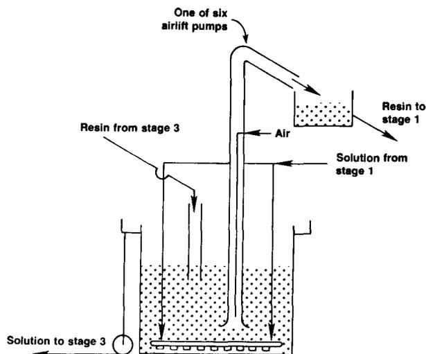
Fig. 2—The Porter CIX contactor
