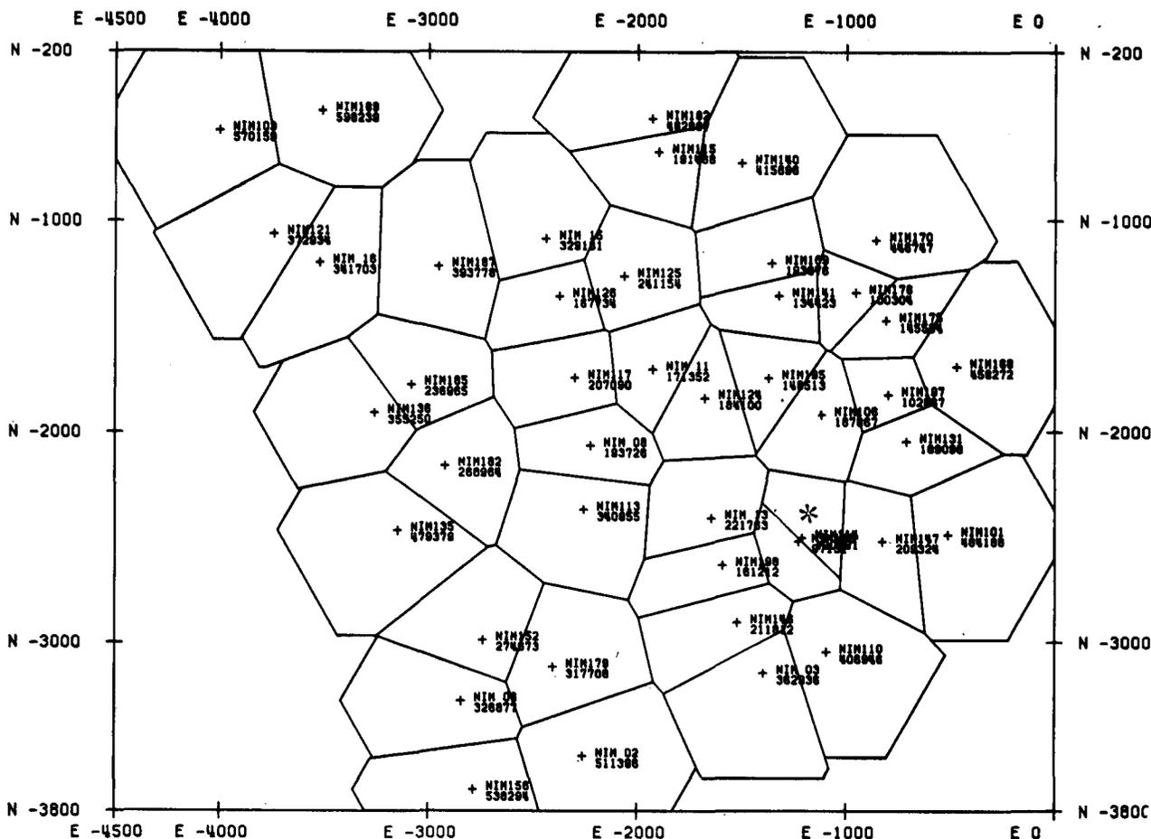
Fig. 4—The polygon areas for the high-yield area, Van der Merwe farm (scale 1:20 000)
