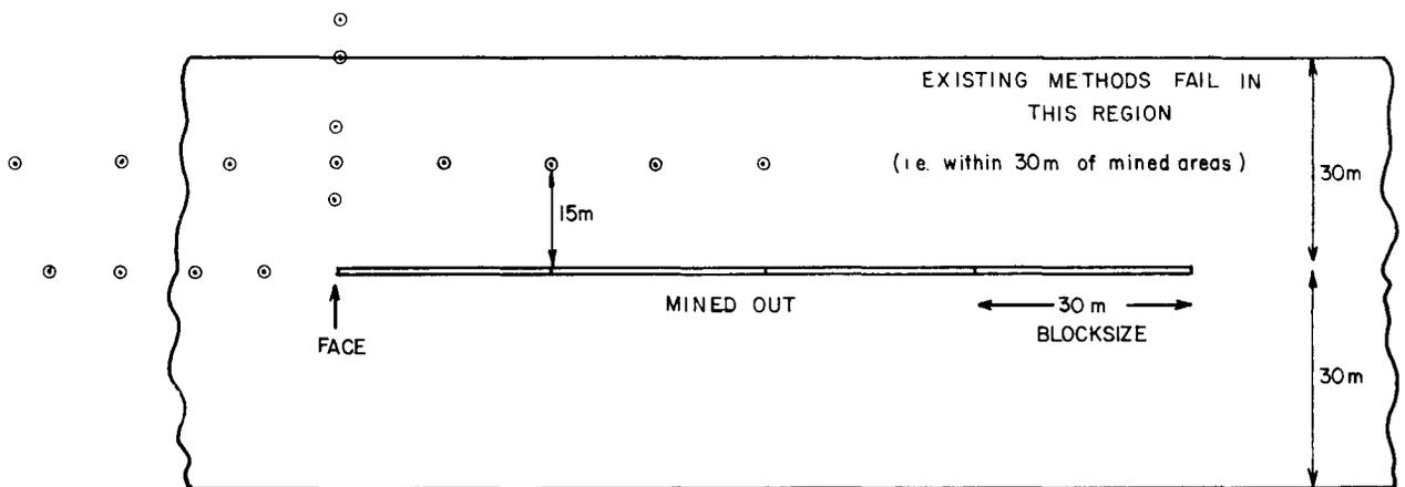
Fig. 1—Points at which stresses and displacements were calculated in an assumed slope 120 m wide with a blocksize of 30m
