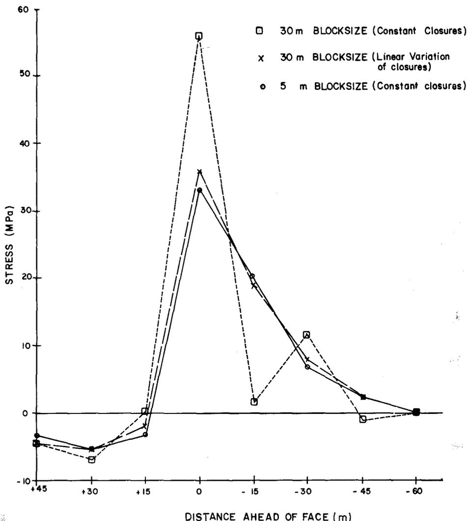
Fig. 3—Shear stresses 15m above the excavation
