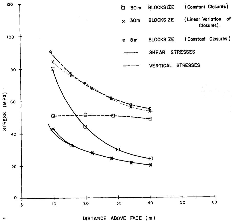
Fig. 4—Vertical and shear stresses directly above the face
