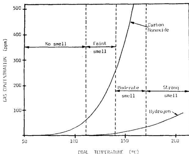
Fig. 1— Development of smell with increase in coal temperature
