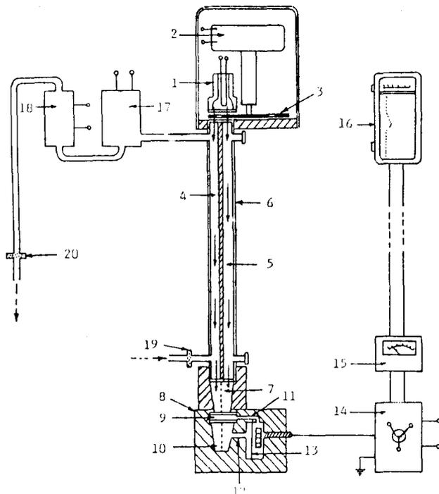
Fig. 2—A typical single-beam infrared gas analyser
