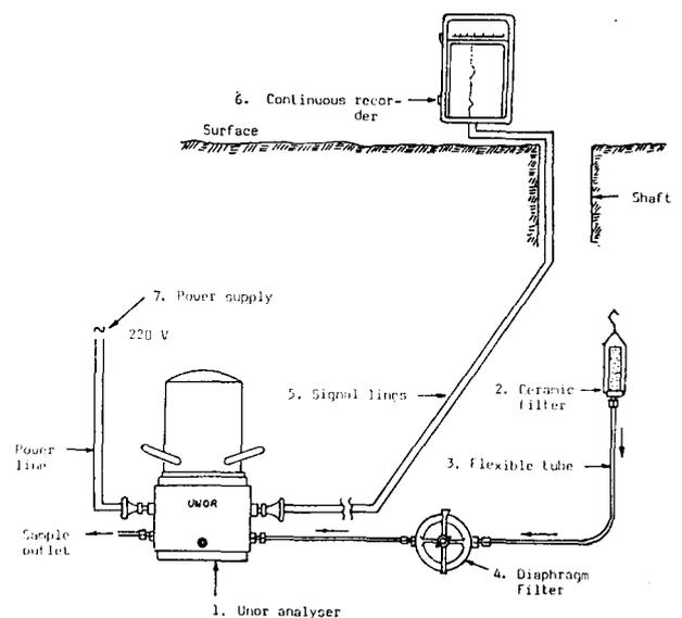
Fig. 5—The telemetric system
