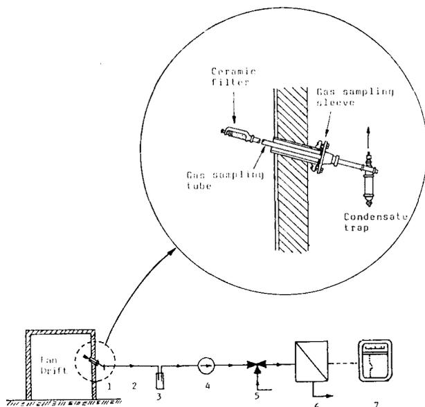
Fig. 6—The upcast-shaft monitor
