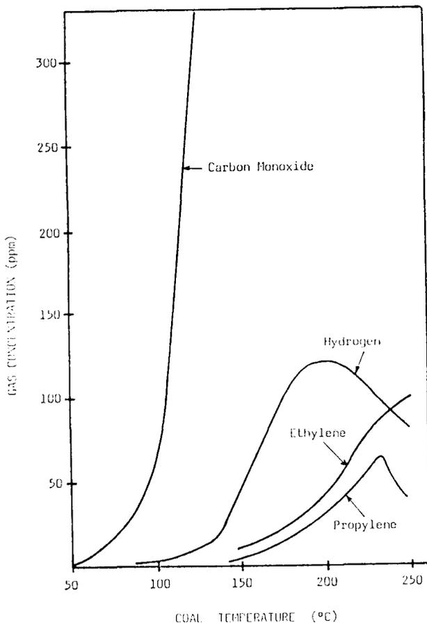
Fig. 3—Gas concentration versus temperature during dynamic non-isothermal oxidation tests with paced heating
