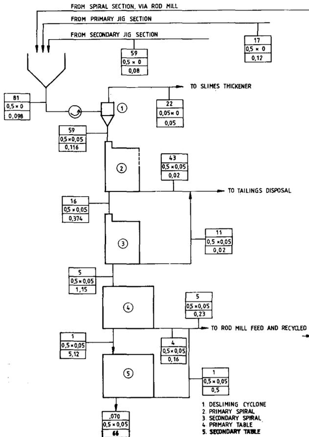
Fig. 3—The spiral section at the Uis Mine
