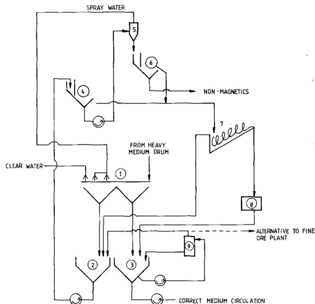
**Fig. 9—The dilute-medium circuit of the heavy-medium separation plant (coarse-ore) at Sishen Mine, South Plant**
