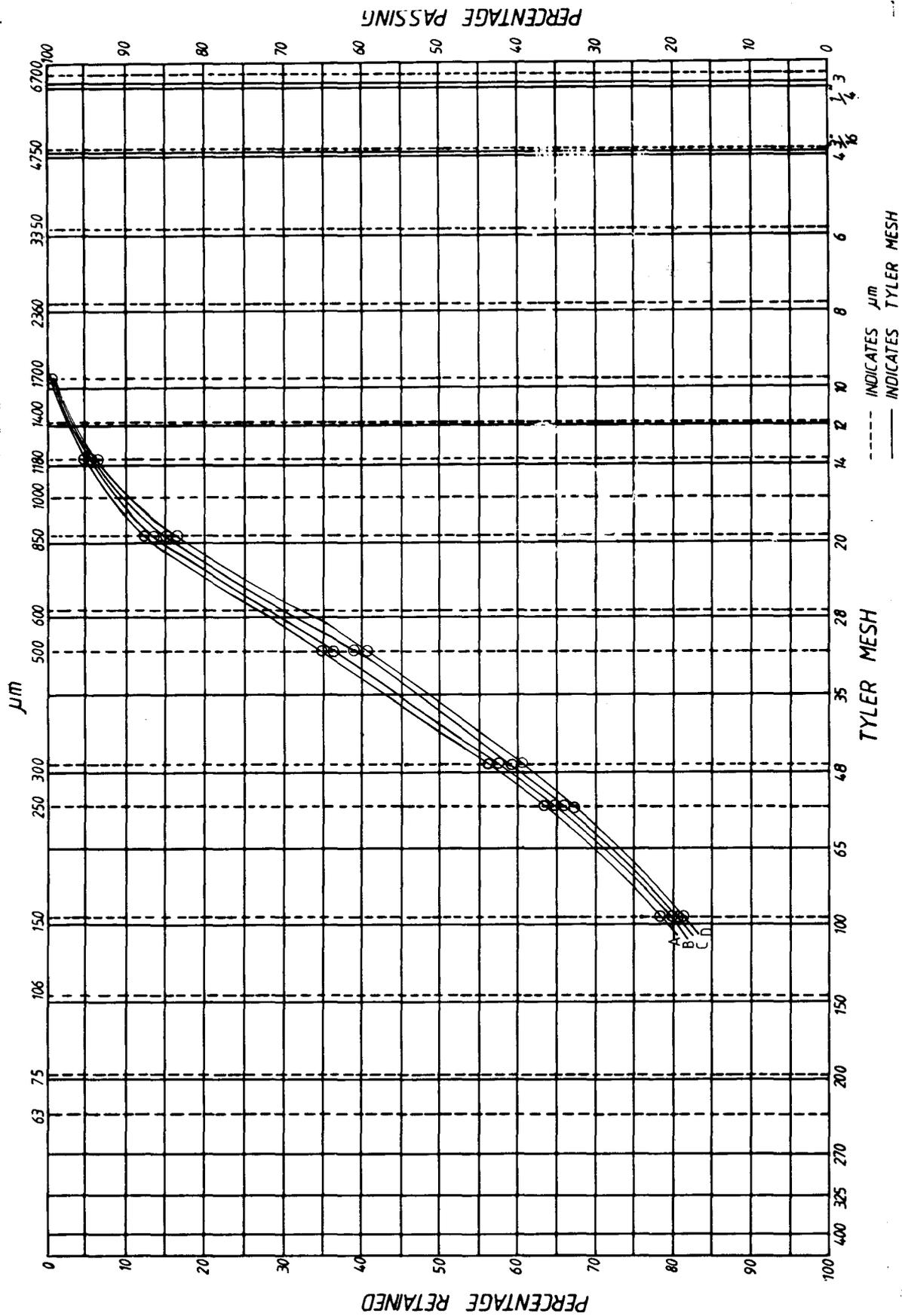
Fig. 5—The size grading of the feed to the secondary distributors after modification of the primary collector box and distributor
