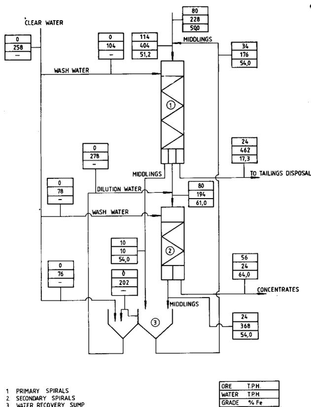
Fig. 6—The fine-ore beneficiation plant at Thabazimbi Mine—the spiral section from the feed-preparation screens
