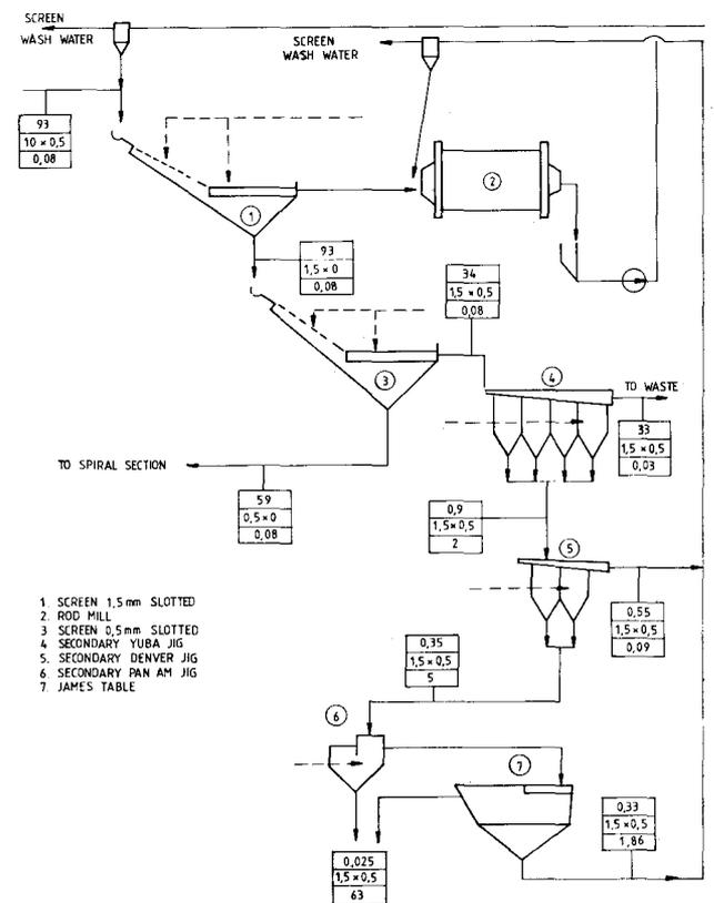
Fig. 2.—The rod-milling and secondary jigging section at the Uis Mine
