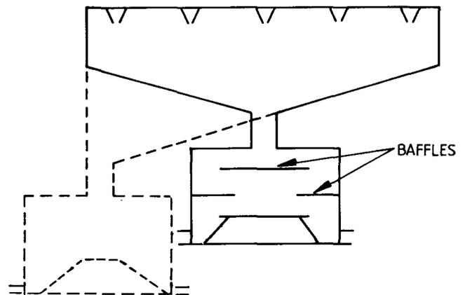
Fig. 4—The modified primary collector box and distributor (the broken line shows the original design)
