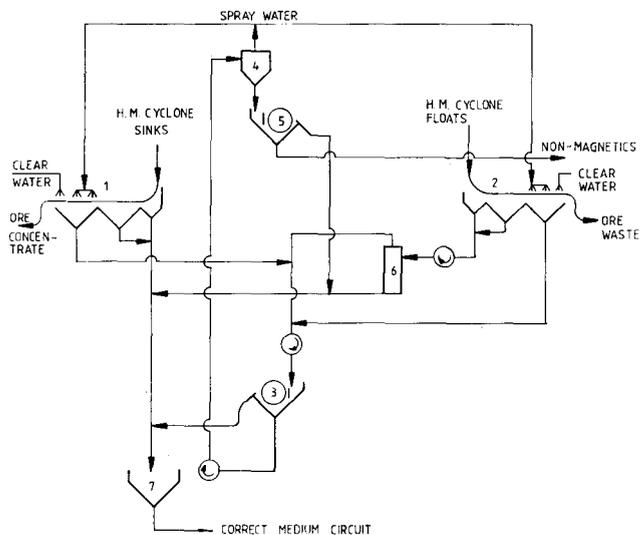
**Fig. 8—The dilute-medium section of the fine-ore beneficiation plant at Thabazimbi Mine**
