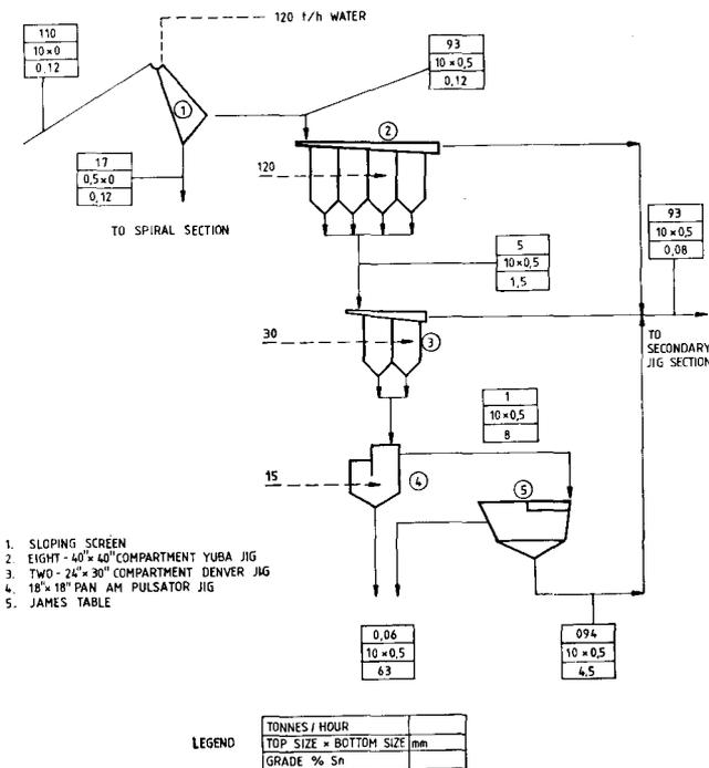
Fig. 1.—The primary jigging section at the Uis Mine
