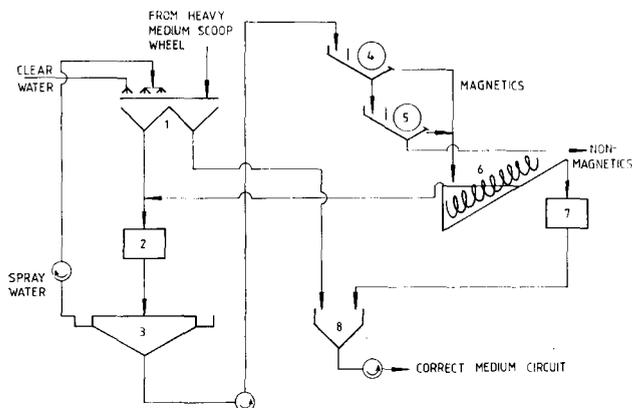
**Fig. 7—The dilute-medium circuit of the heavy-medium separation plant (coarse ore) at Thabazimbi Mine**
