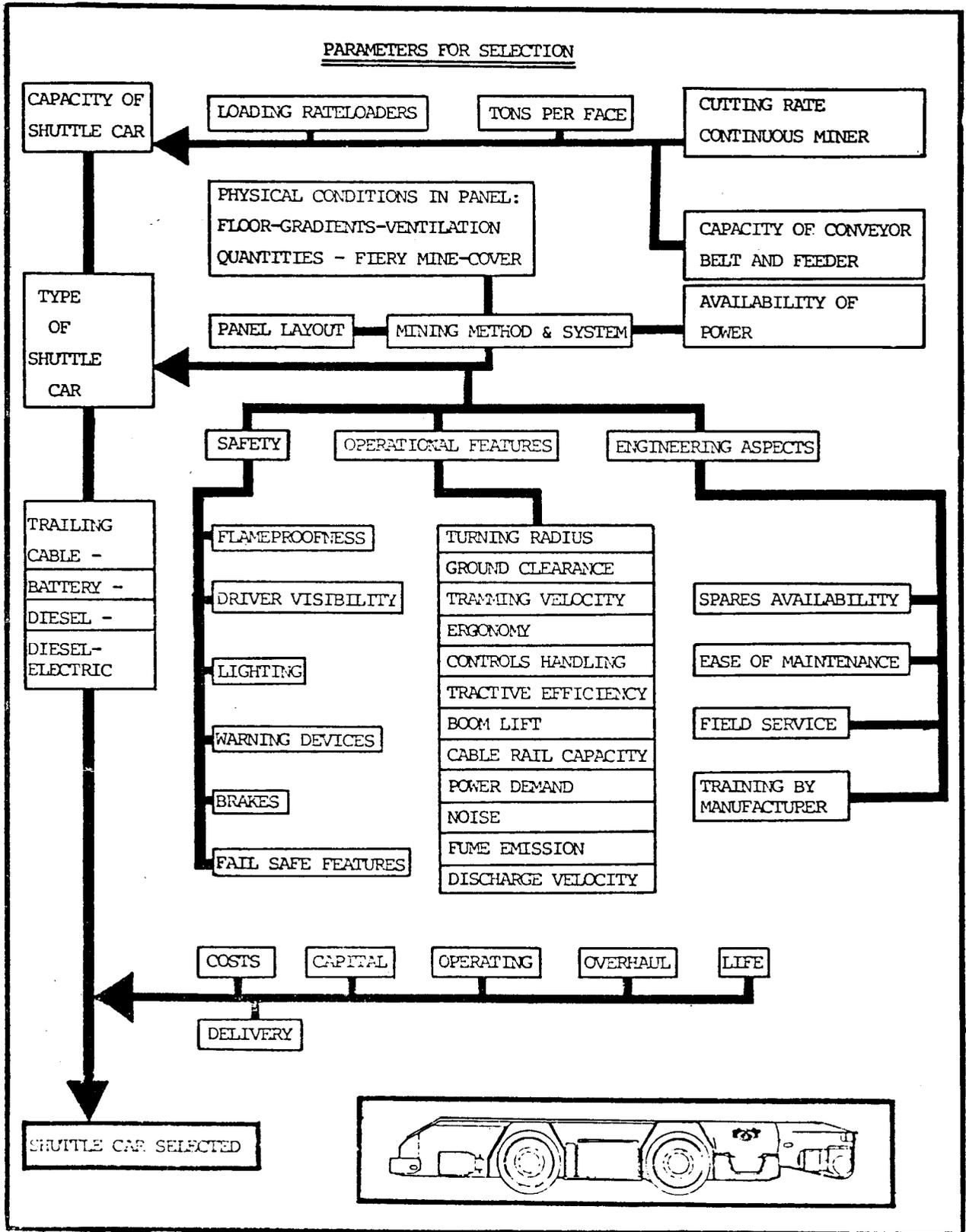
Fig. 3—Criteria for the selection of a shuttlecar
