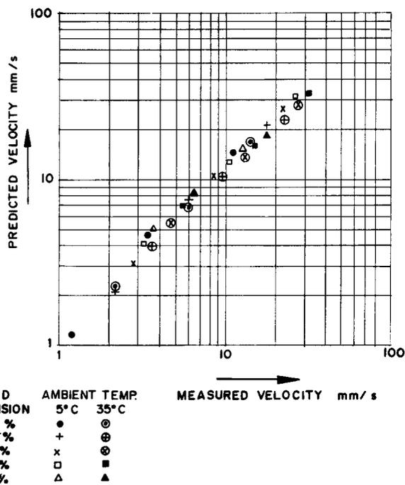
Fig. 3—Hindered settling velocities of wetted activated carbon (relative density 1,28) in water (measured velocities from Edward L. Bateman).
