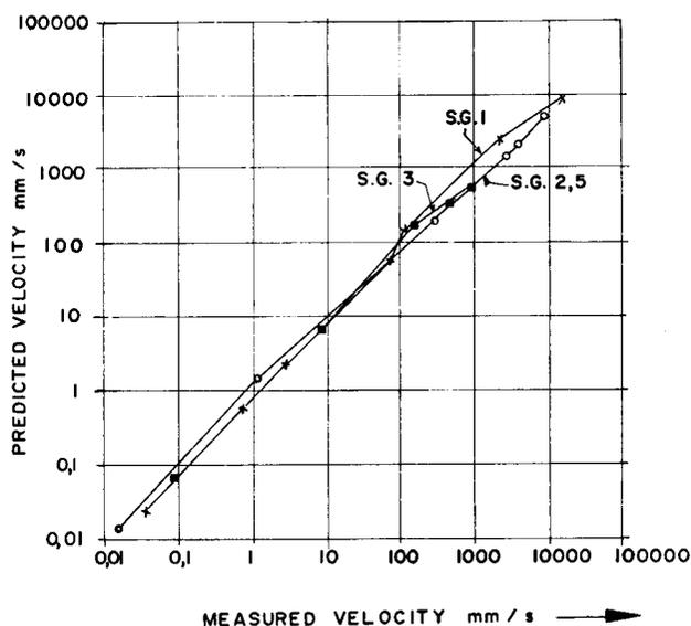
Fig. 2—Free settling velocities in air (measured velocities from Taggart<sup>2</sup>). SG = specific gravity or relative density.
