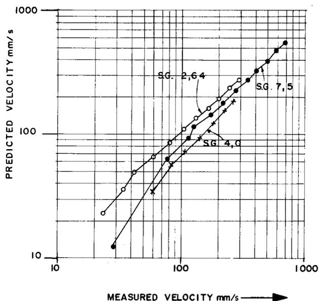
Fig. 1—Free settling velocities in water (measured velocities from Taggart<sup>1</sup>). SG = specific gravity or relative density.
