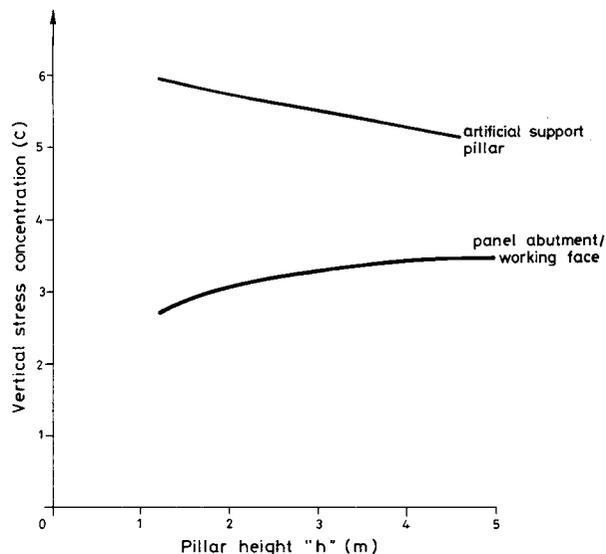
Fig. 4—Effect of pillar height,  $h$ , on the stress concentration at the internal support pillars and the panel abutment. The depth of mining is 100 m, the panel width 200 m, and the reloading modulus of the material 1 GPa.
