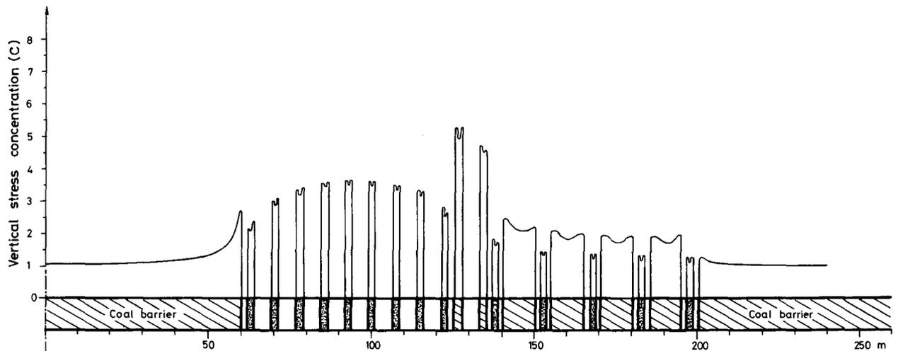
**Fig. 5—Vertical stress concentration around an existing bord-and-pillar panel in which pillars are extracted according to the concept of artificial support pillars. The depth of mining is 100 m, the seam thickness 1,8 m, and the modulus of compression of the pillar material 1 GPa.**
