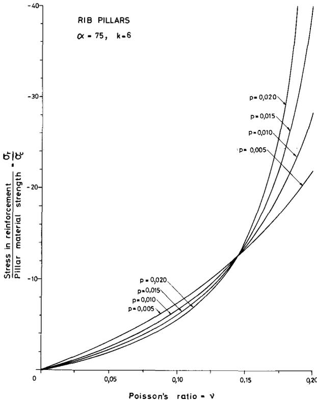
Fig. 4—Tensile stress in the reinforcement
