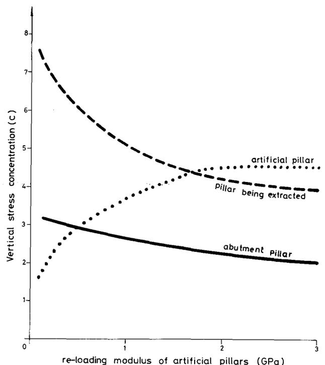
**Fig. 6—Effect of the modulus of compression on the stress conditions in pillar-extraction panels employing artificial support pillars. The depth of mining is 100 m, the extracted span 60 m, and the mining height 1,8 m.**
