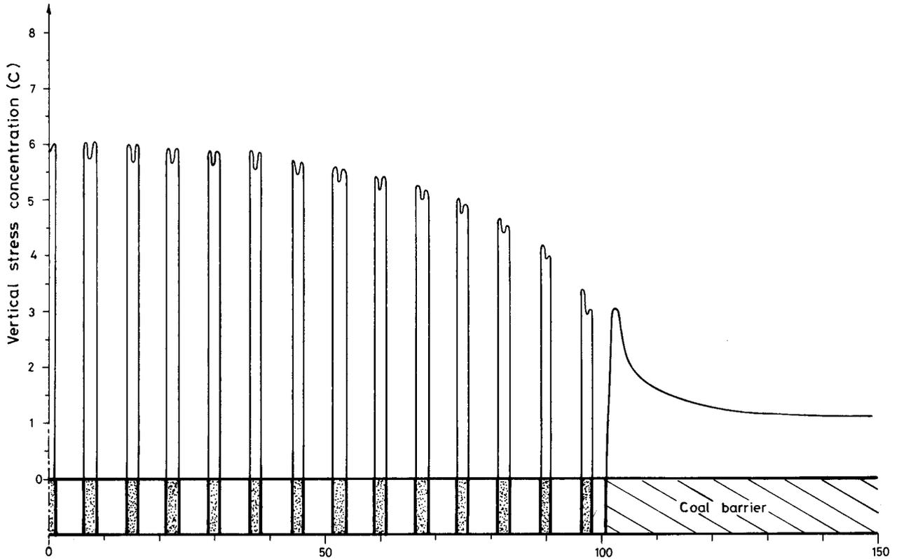
**Fig. 1—Stress distribution around a 200 m-wide total extraction panel situated at a depth of 100 m. The panel is supported by artificial pillars that are constructed from a material with a modulus of compression of 1 GPa. Because the panel is symmetrical, only the right-hand side is shown.**
