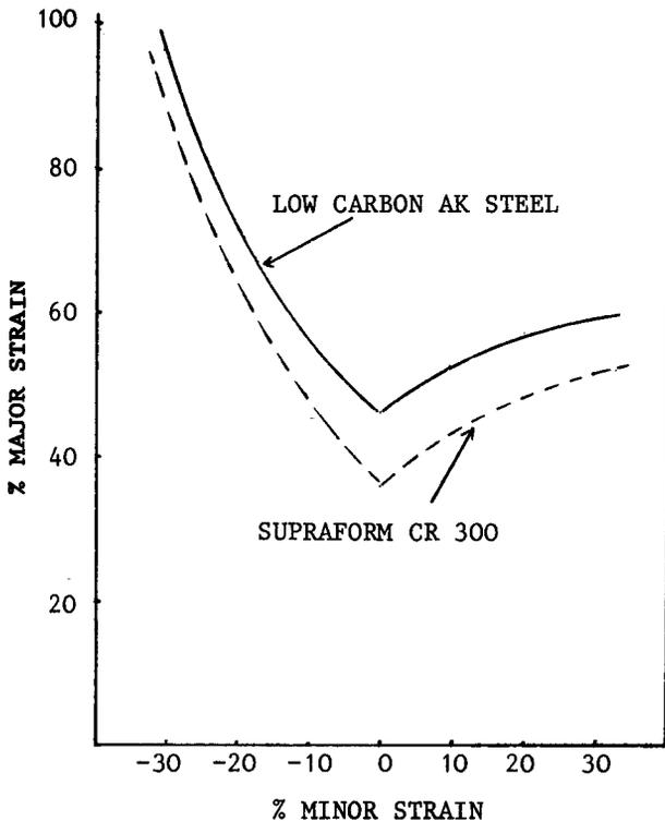
Fig. 2—Probability limits for 1,6 mm material
