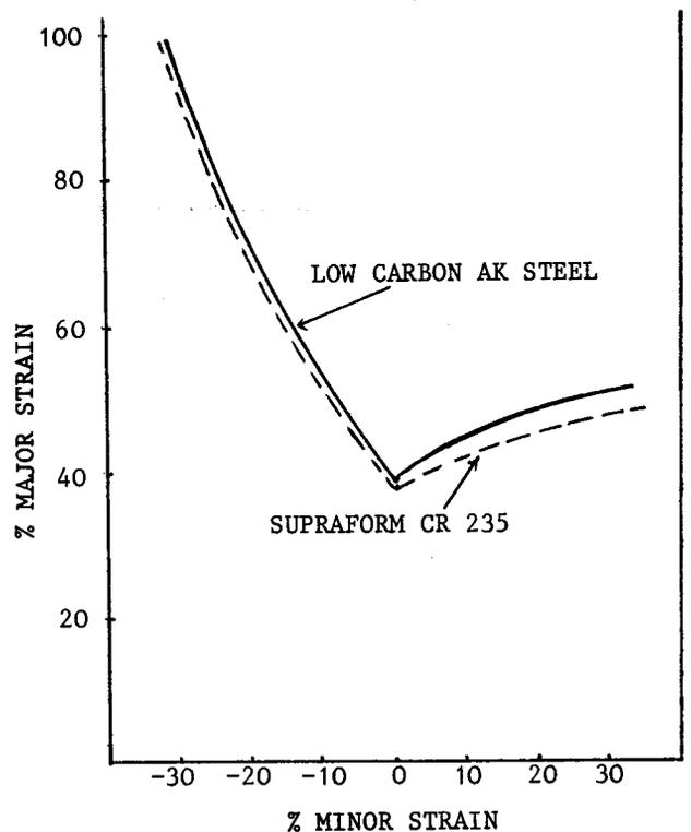
Fig. 1—Probability limits for 1,0 mm material
