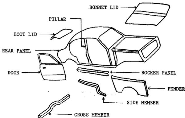
Fig. 4—Autobody parts from HSCR steels
