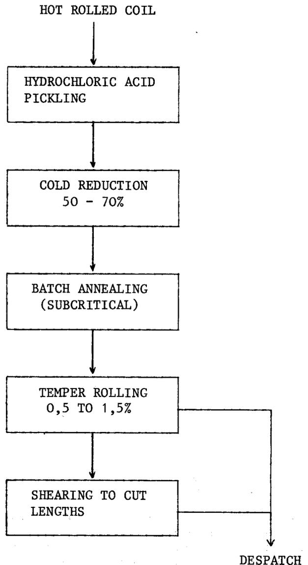
Fig. 3—Production flow for cold-rolled products
