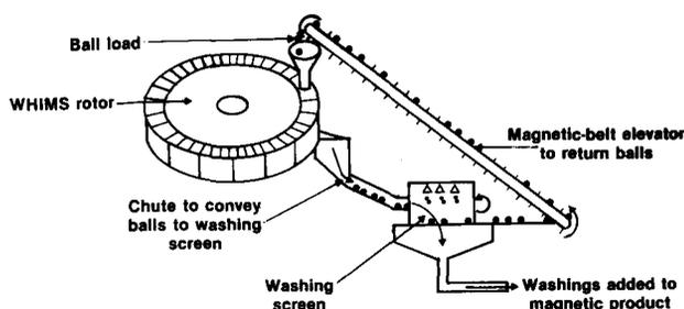
Fig. 4—The WHIMS rotor, showing the system for cleaning and returning the balls
