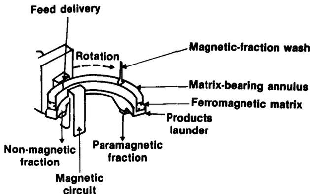
Fig. 3—Schematic representation of a WHIMS machine
