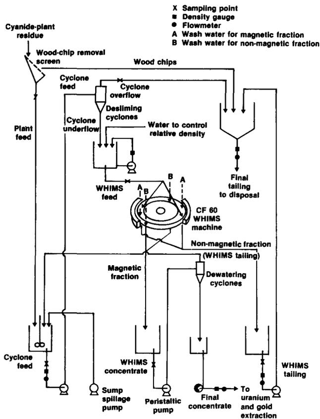
Fig. 1—Flowsheet of the WHIMS installation at a gold mine
