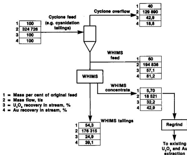
Fig. 6—Mass flow and recoveries on a gold mine
