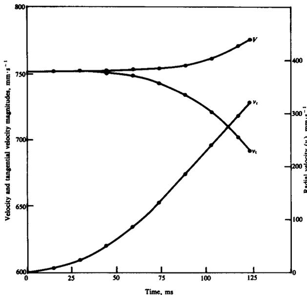
Fig. 7—Calculated time dependence of the magnitudes of the rod velocity ( $V$ ) and of its radial ( $v_r$ ) and tangential ( $v_t$ ) components during the interaction between the rod and lifter bar. At about 29 ms after equilibrium,  $v_t$  passes through a maximum.
