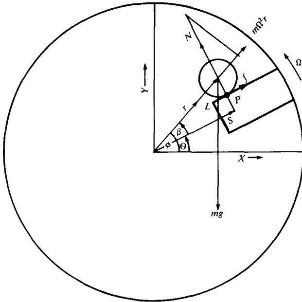
Fig. 4—A dynamic model of the sliding interaction. The diagram exaggerates the sizes of the rod and the lifter bar relative to that of the mill, and shows that angle  $\beta$  is a function of the rod position on the lifter bar.
