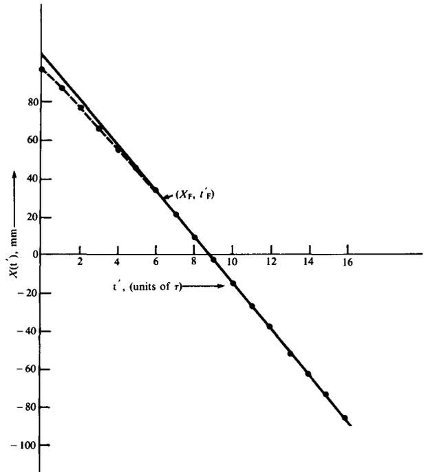
Fig. 3—The measured dependence of the  $X$  coordinate of the rod position on time  $t'$ . The dependence is linear for  $t' > 7\tau$ . The departure from linearity at shorter times indicates that there was an interaction between the rod and the lifter bar in the angular range B to C, shown in Fig. 2.
