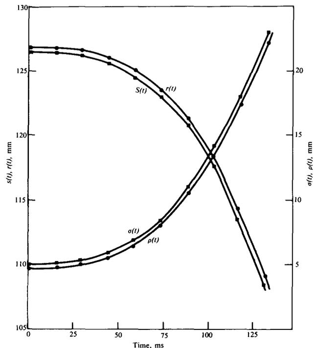
Fig. 5—Time dependence of the displacement of a rod while it is in contact with a lifter bar;  $s(t)$  and  $r(t)$  are measured from the axis, and  $\sigma(t)$  and  $\rho(t)$  from the inner lining.
