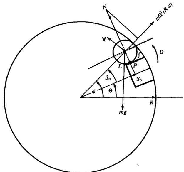
Fig. 1—Interaction of a rod and a lifter bar. The sizes of the rod and the lifter bar relative to the mill have been exaggerated to reveal that, when the lifter bar is at angle  $\theta$ , the rod is at angle  $\phi$  and the normal reaction  $N$  has a component along the radius vector through the rod centre.  $P$  is the point of contact between the rod and the surface of the lifter bar, and  $L$  is the edge of the lifter bar.
