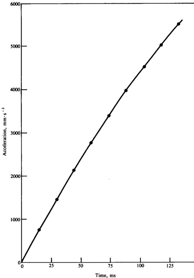
Fig. 6—Time dependence of the magnitude of acceleration of a rod down the surface of a lifter bar.
