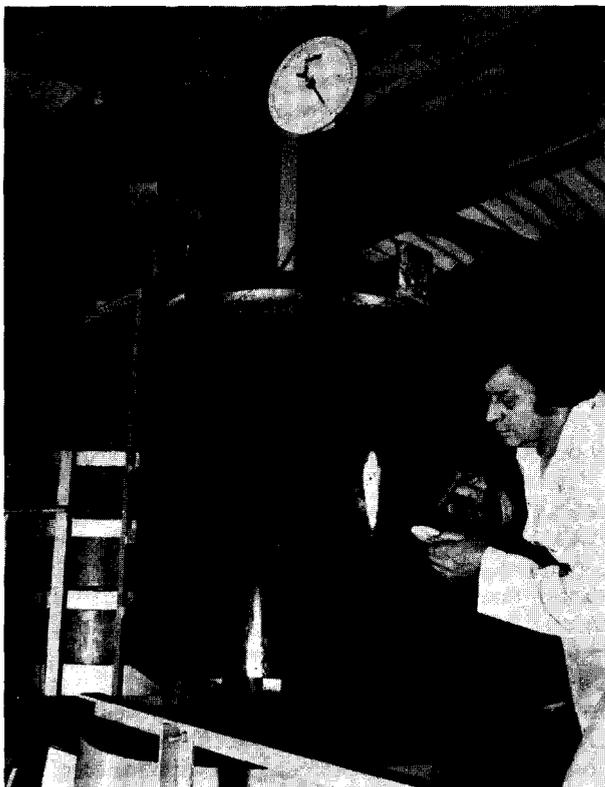
been developed by a British company. In the accompanying photograph, a sample of the silver flake is being collected from a giant cathode in the process that leaves only trace levels of the metal. Depending on through-put, the makers claim that the totally enclosed process can be self-financing and adapted to customers' requirements.
