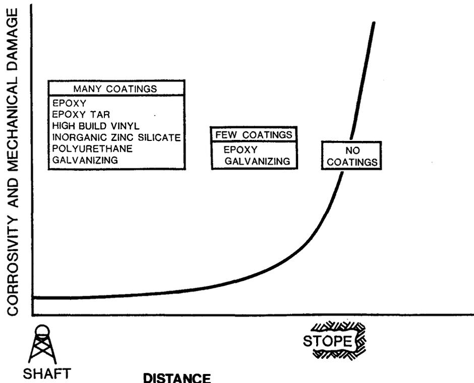
Fig. 3—The suitability of coatings for pipes in gold mines
