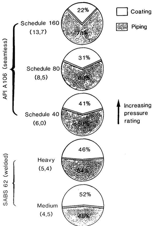
Fig. 4—Variation in the costs of coatings and pipes with increasing pressure rating (the figures in brackets represent pipe wall thickness in millimetres)
