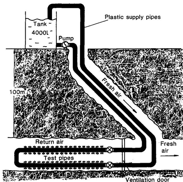
Fig. 1—Schematic layout of the test site
