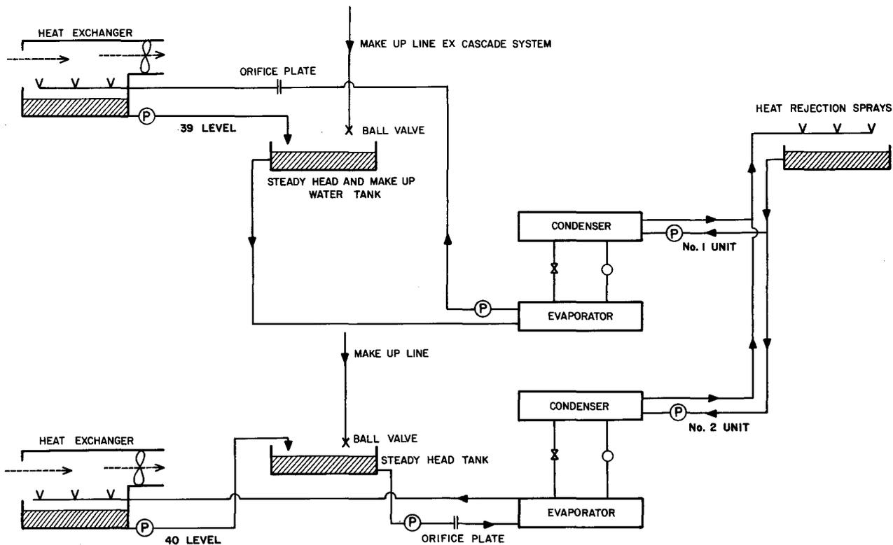
Fig. 2—A schematic diagram showing the cooling system
