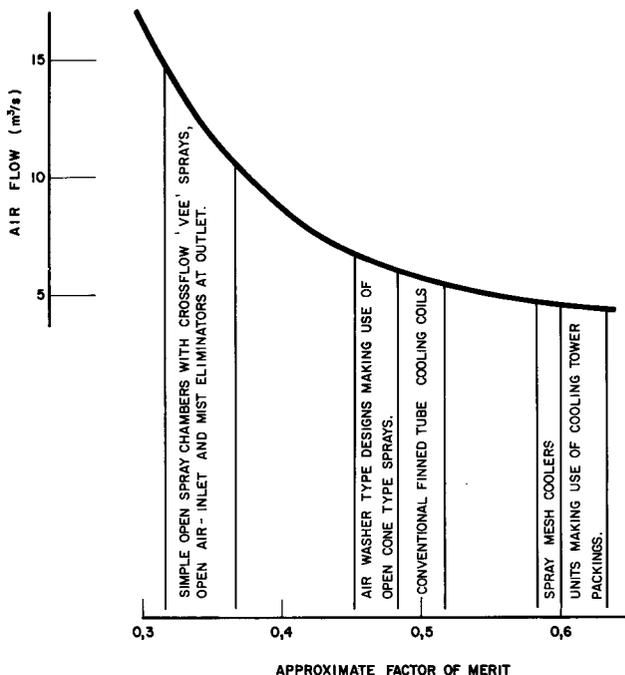
Fig. 4—Required flowrate of air through air coolers of different designs
