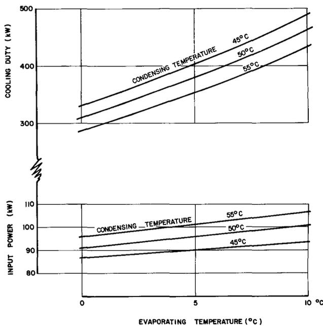
Fig. 3—The expected performance of the refrigeration unit
