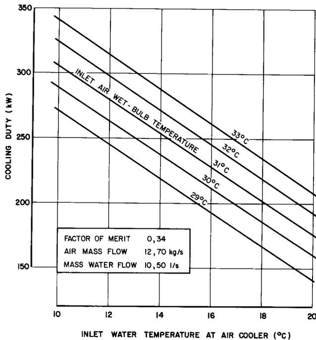
Fig. 5—The expected performance of the air cooler under underground conditions
