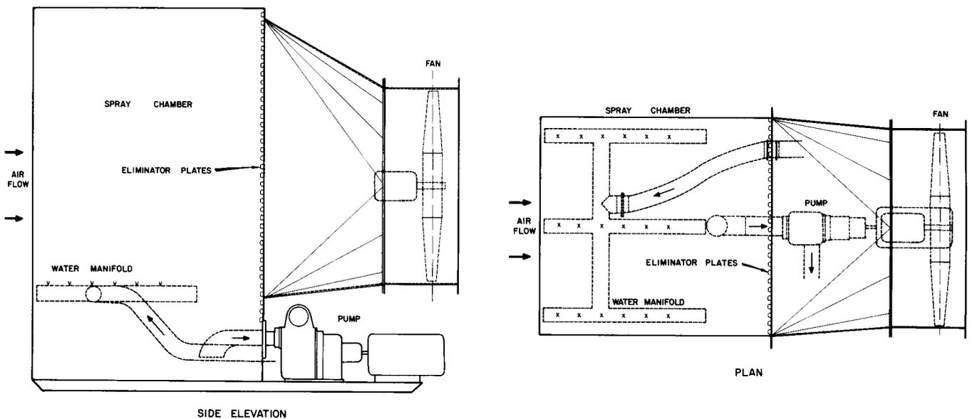
Fig. 6—The final design of the cross-flow air cooler
