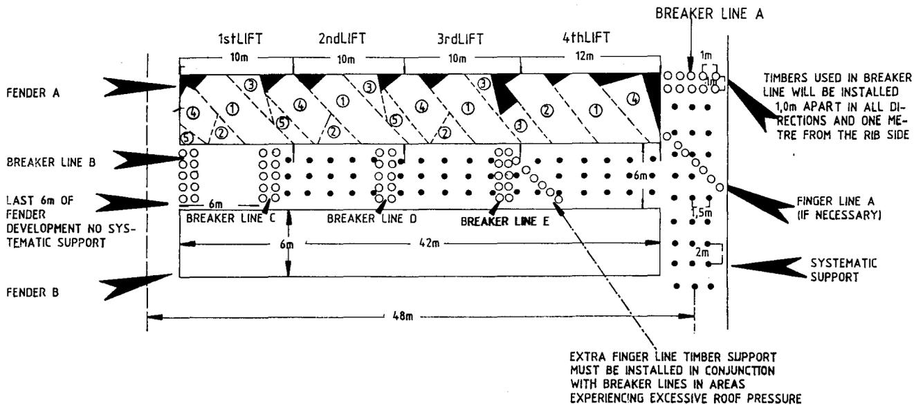
Fig. 8—Diagram showing the systematic support and sequence of the cutting used in rib pillar extraction
