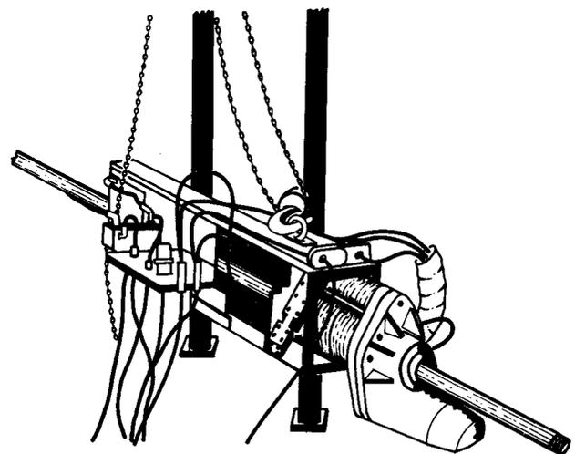
Fig. 2—A horizontal diamond drill
