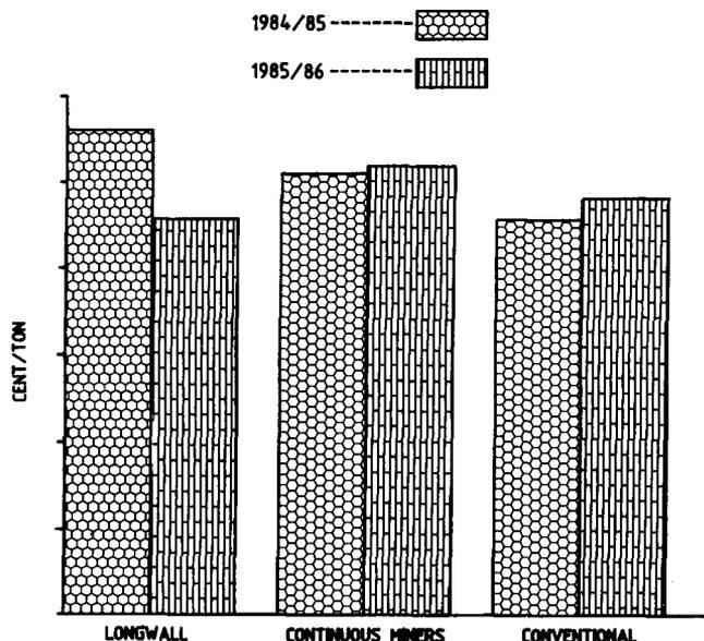
Fig. 5—Relative production costs for the longwall, continuous-miner, and conventional units
