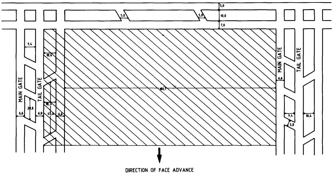
Fig. 6—Mining of an interpanel pillar at Secunda Collieries
