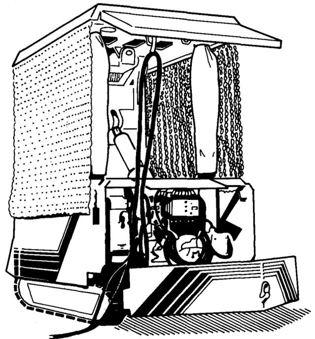
Fig. 7—Breaker-line support
