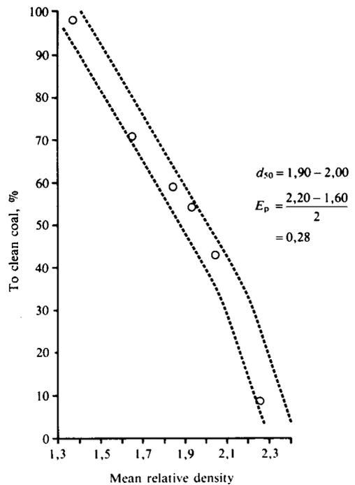
Fig. 3—Partition factors in laboratory froth flotation at the University of Natal<sup>12</sup>
