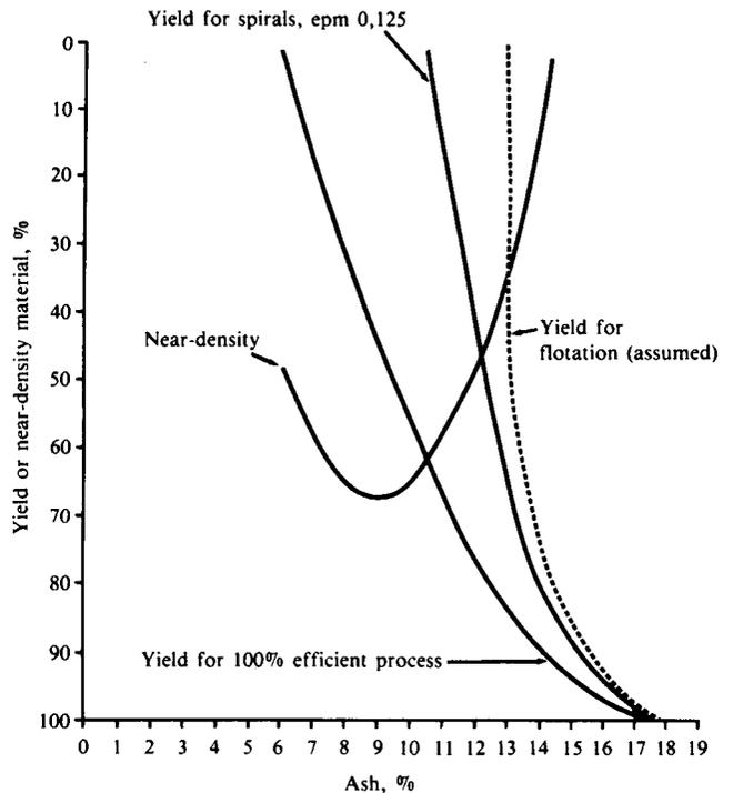
Fig. 2—Flotation results under identical conditions of reagents, concentrations, etc.
