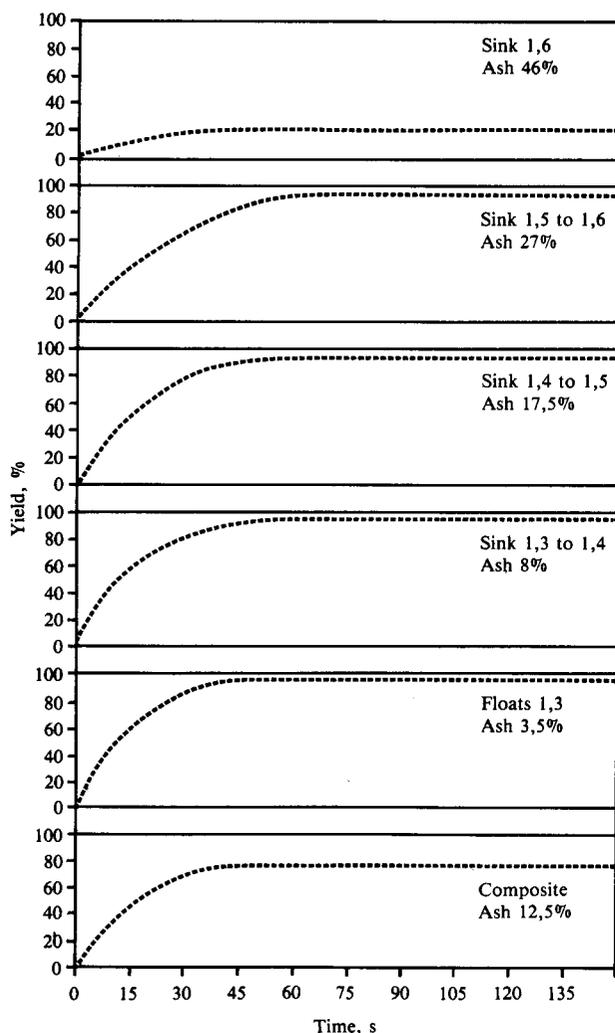
Fig. 1—Liberation of various fractions in froth flotation at the same dosage of reagent<sup>1,2</sup>
