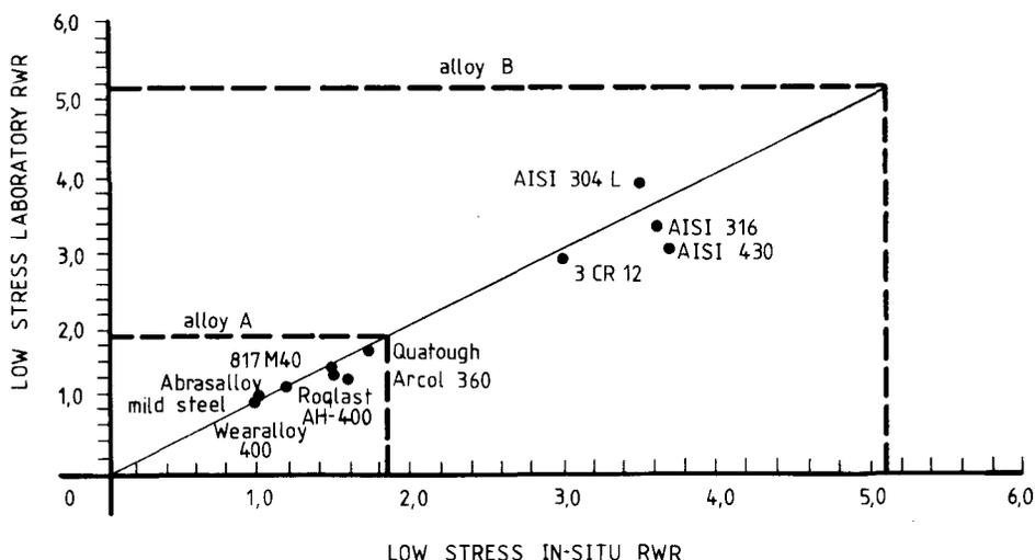
by the appropriate manipulation of chemical compositions, and fabrication procedures. A concept of microstructural design was therefore employed in the development of a series of alloys with a hardness of more than 500 VPN and an impact toughness of more than 30 J.
