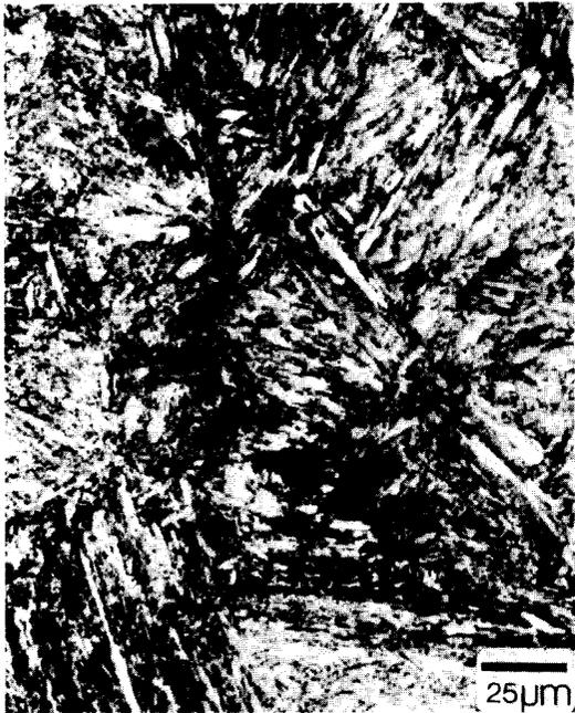
Fig. 2—General structure of alloy A (optical)
