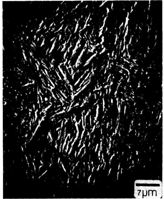
Fig. 3—Martensite morphology of alloy B (SEM)
