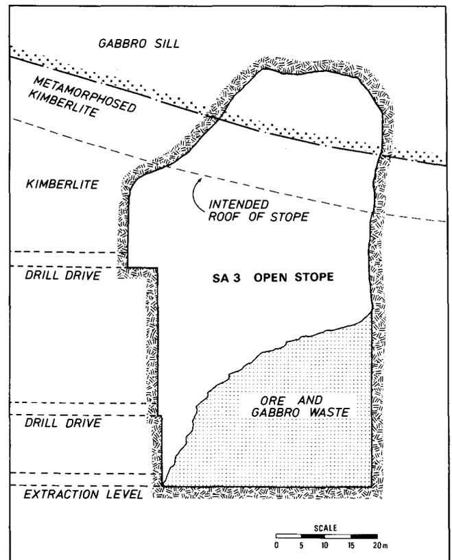
Fig. 4—Extent of the collapse of the gabbro sill into the SA3 stope
