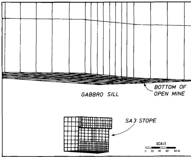
Fig. 5—Three-dimensional boundary-element model of the SA3 stope
