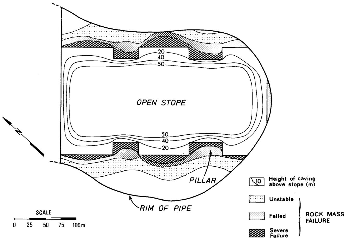
Fig. 9—Plan showing the predicted failure of the rock mass and the height of caving above the stope roof with reduced lead between stopes and pillars
