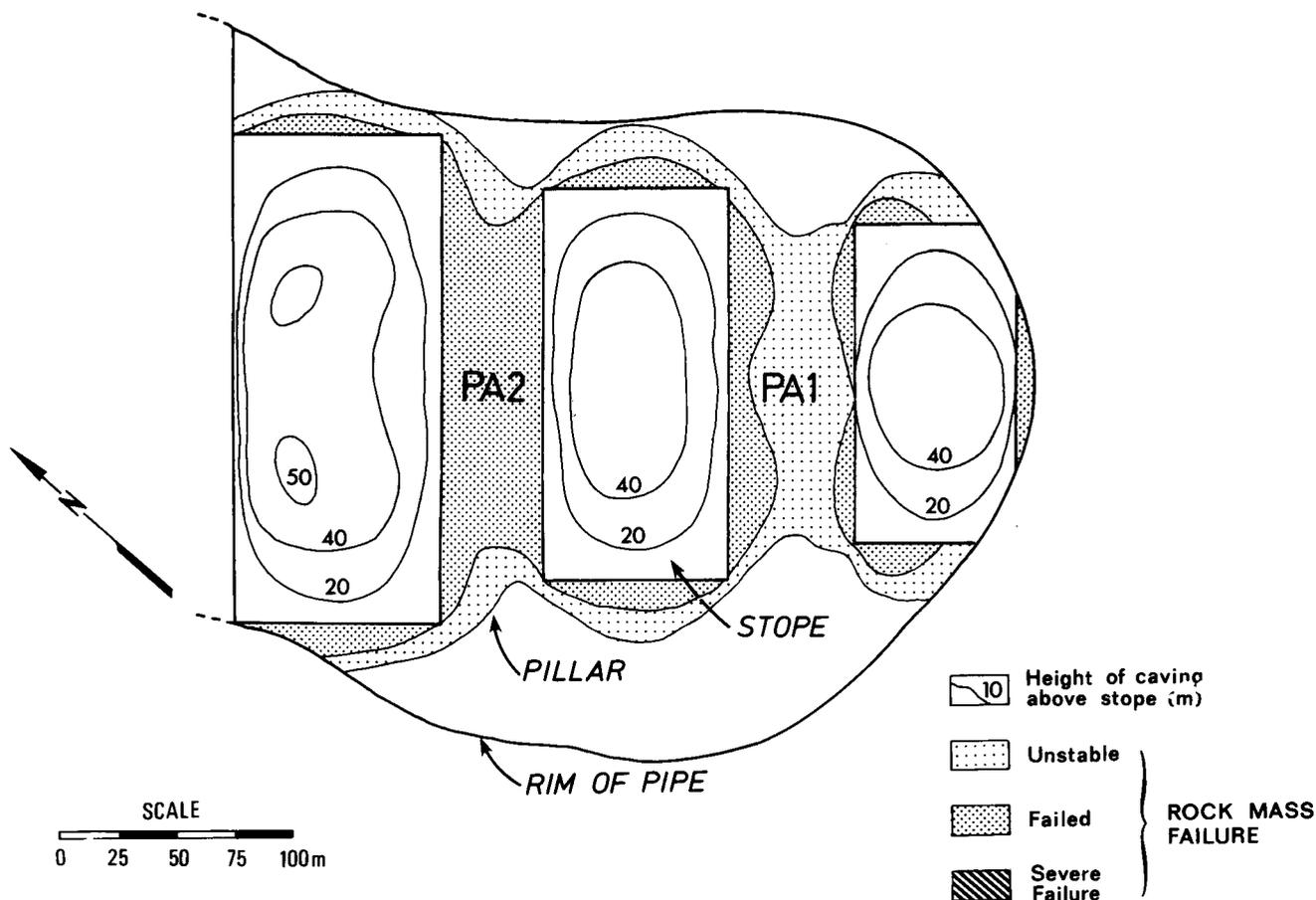
Fig. 7—Plan showing the predicted failure of the rock mass and the height of caving above the stope roof
