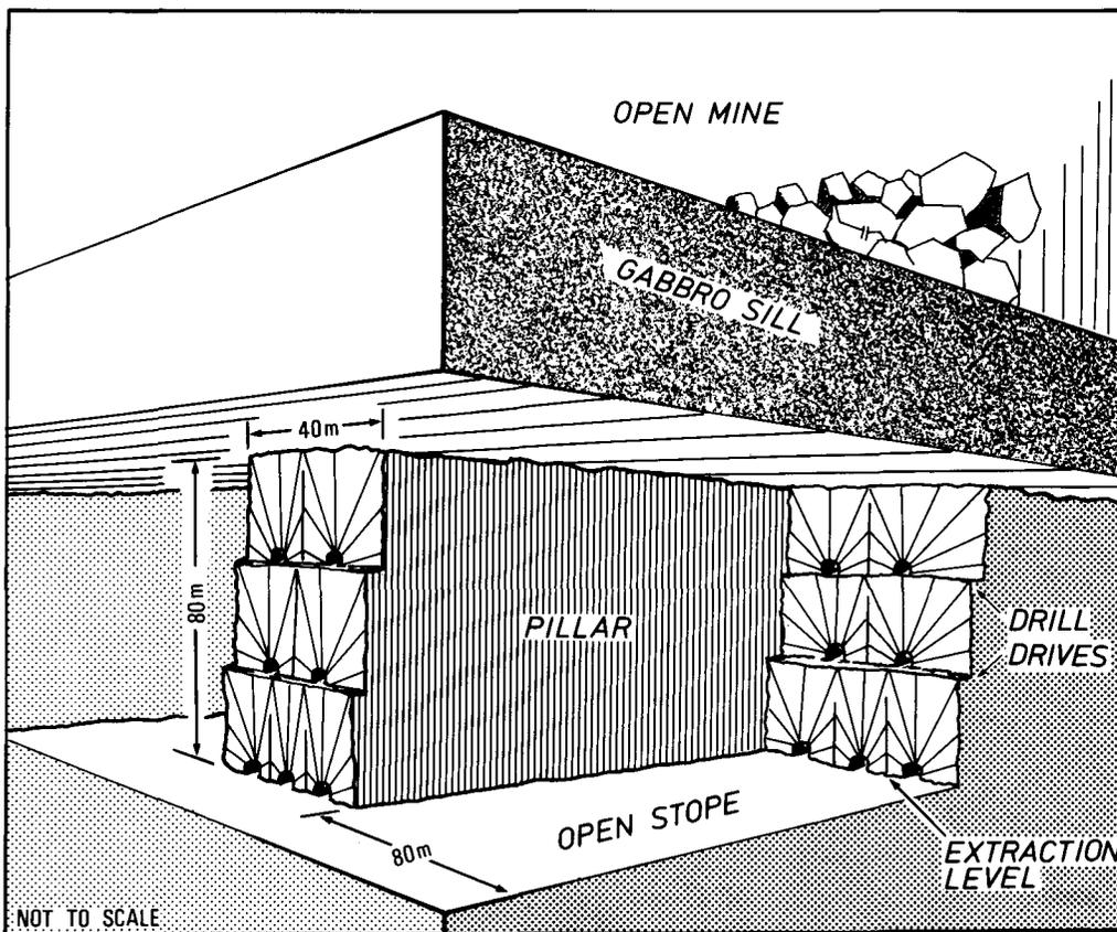
Fig. 1—Layout of the open stopes and pillars beneath the gabbro sill
