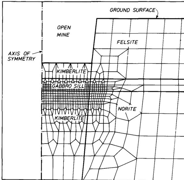
Fig. 3—Finite-element model of the mine
