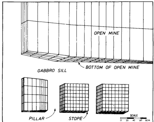
Fig. 6—Three-dimensional model of the open stopes prior to pillar extraction
