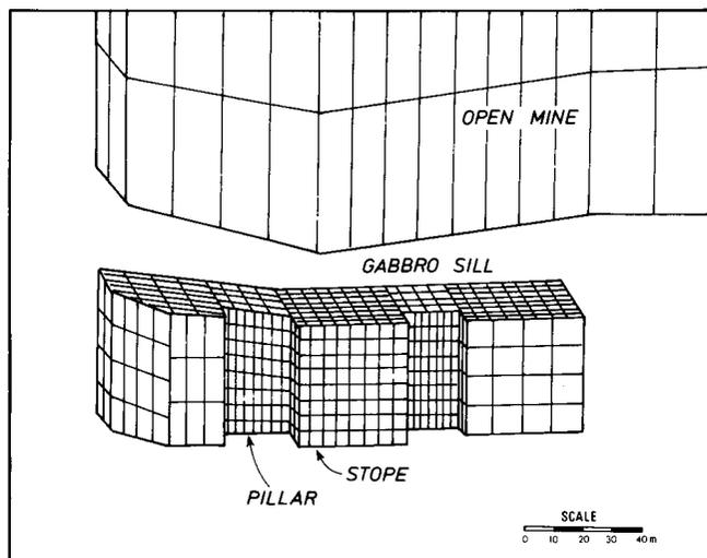
Fig. 8—Three-dimensional model of stopes and pillars during pillar extraction
