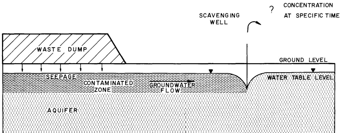
Fig. 1—Illustrative system for the prediction of seepage quality at a scavenging well
