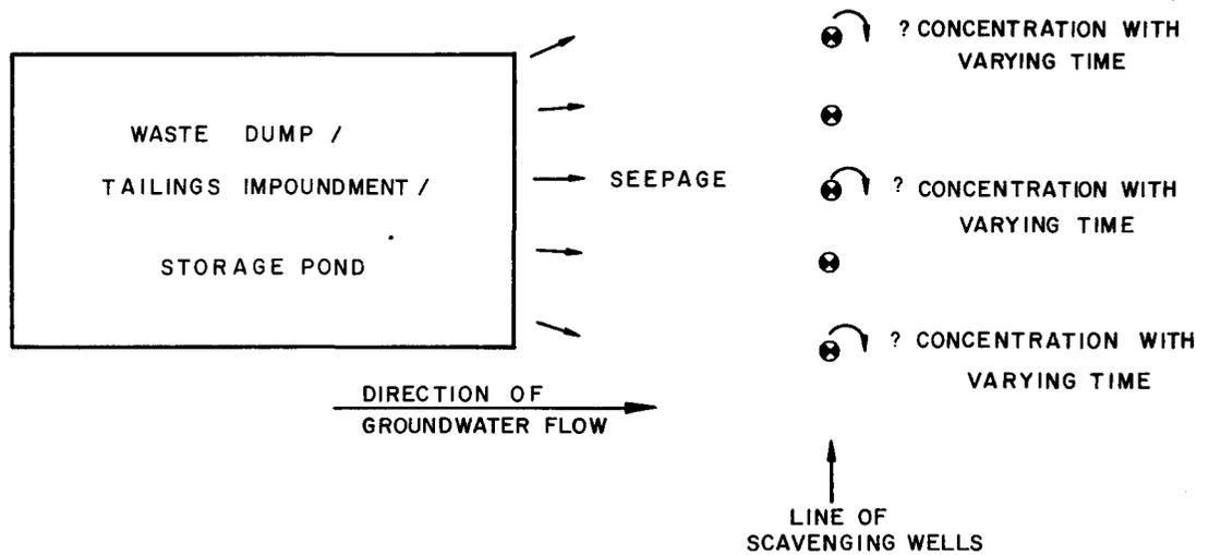
Fig. 4—Model 2: A two-dimensional (plan) solute-transport model—AQUISOL
