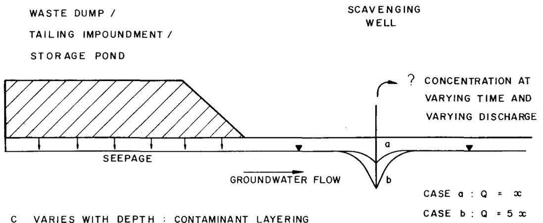
Fig. 5—Model 3: A two-dimensional (sectional) solute-transport model—QSOL
