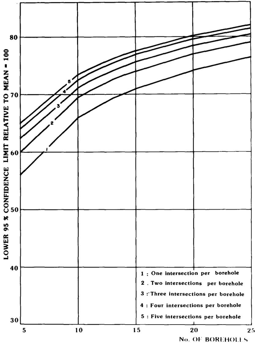
Fig. 12—Lower 95 per cent confidence limit for the Basal Reef (mean = 100)
