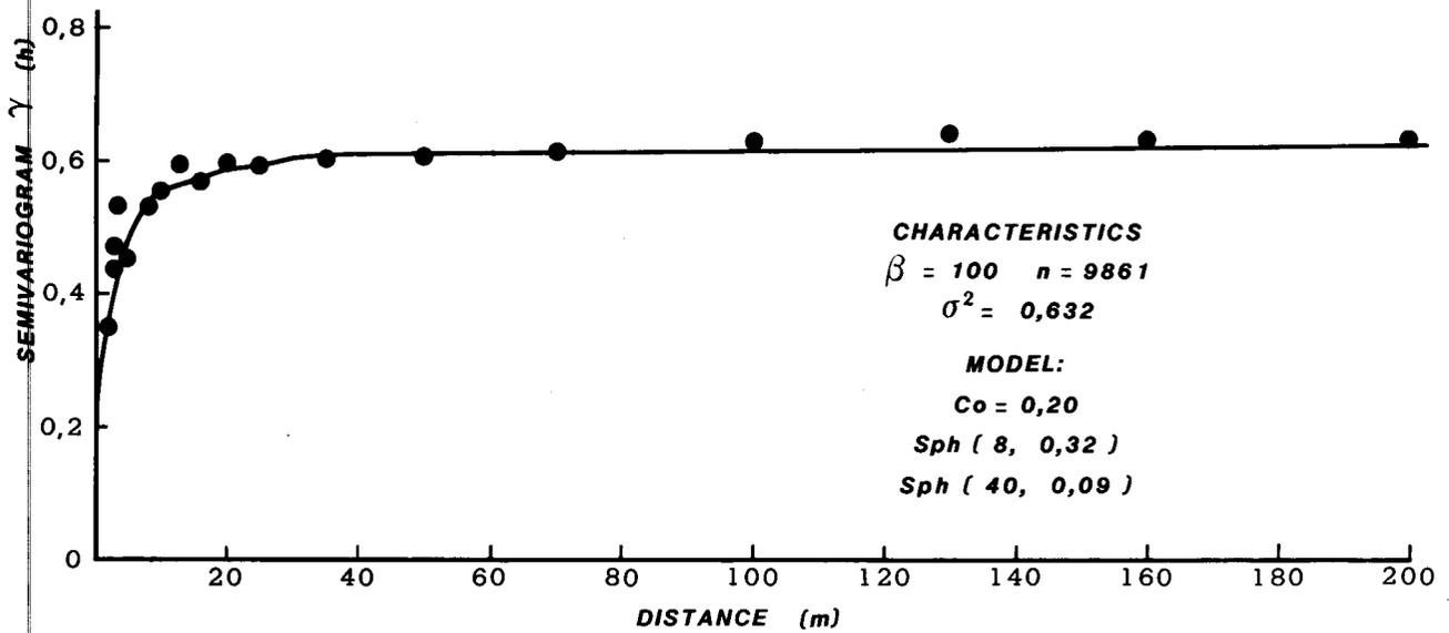
Fig. 3—Semi-variogram of the Basal Reef
