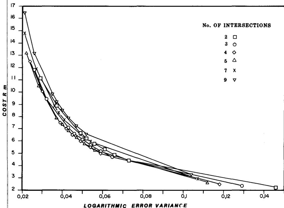
Fig. 16—Analysis of borehole deflections for the Vaal Reef at a depth of 3000 m
