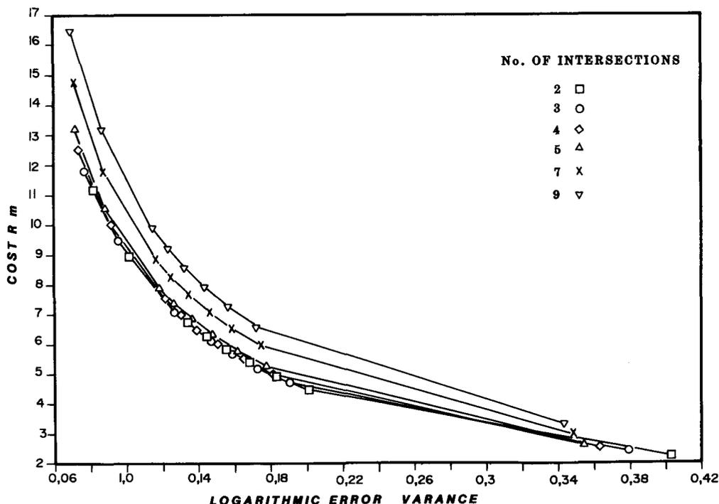
Fig. 17—Analysis of borehole deflections for the Elsburg Reef at a depth of 3000 m
