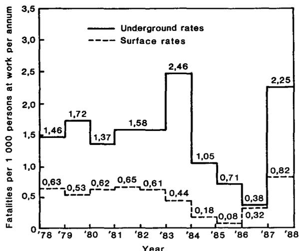
Fig. 2—Underground and surface fatality rates on coal mines belonging to the Chamber of Mines of South Africa (1978–1987)
