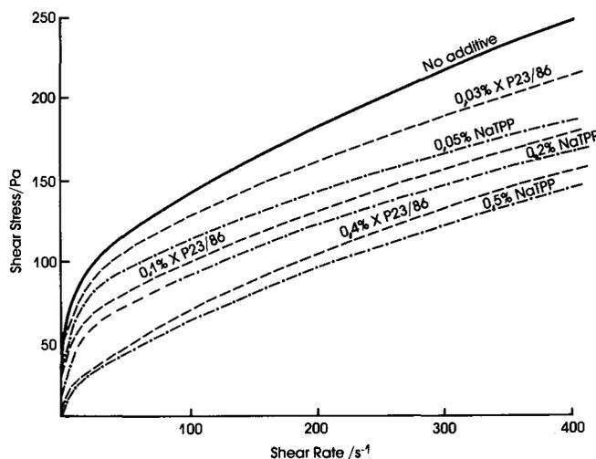
Fig. 2—Shear stress versus shear strain for WAGM tailings at a total solids concentration of 71,4 per cent with increasing amounts of NaTPP (·-·-) or XP23/86 (---)
