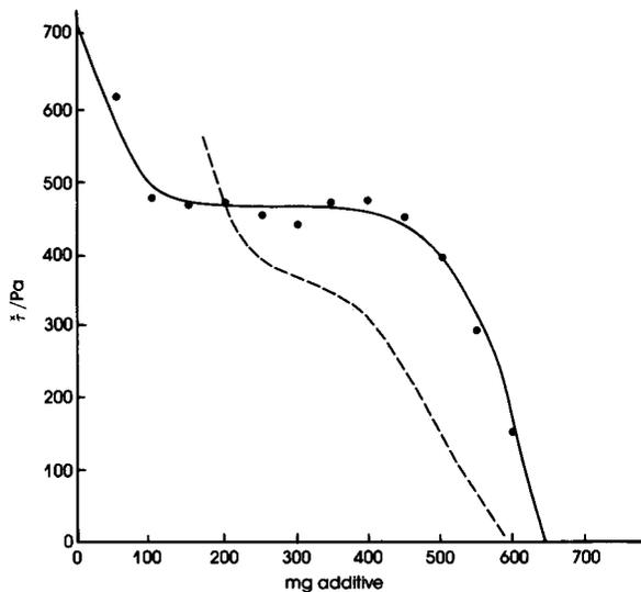
Fig. 5—Variation in flow stress barrier ( $\bar{\tau}$ ) of the  $\text{SiO}_2$ -5%  $\text{Fe}_2\text{O}_3$ - $\text{H}_2\text{O}$  slurry with increasing amounts of NaTPP (— · — · —) and the titration curve of NaTPP (— · — · —)
