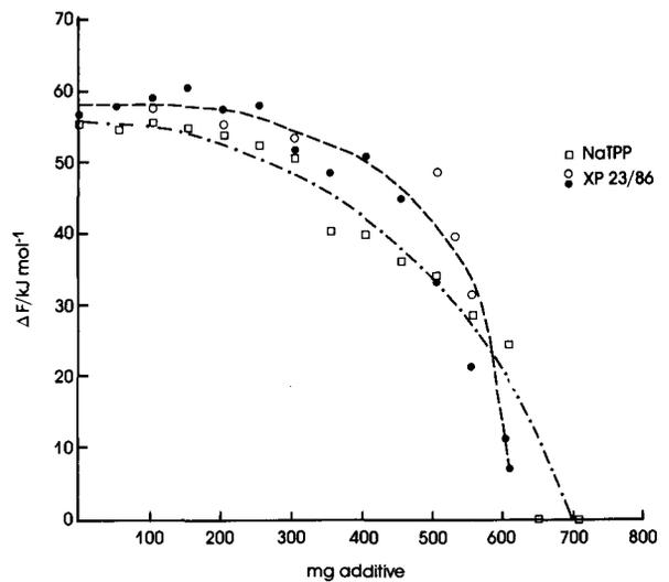
Fig. 3—Variation in flow activation energy ( $\Delta F$ ) of the  $\text{SiO}_2$ -5%  $\text{Fe}_2\text{O}_3$ - $\text{H}_2\text{O}$  slurry with increasing amounts of sodium tripolyphosphate (— · — ·) and XP23/86 (— — —)
