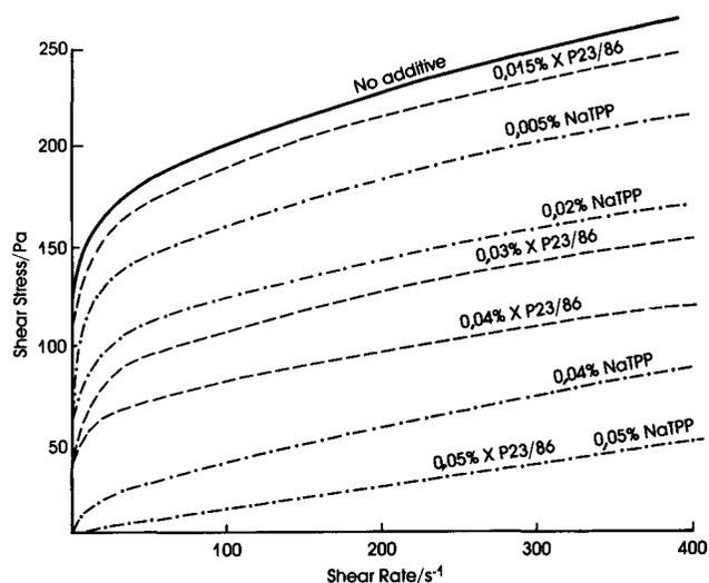
Fig. 1—Shear stress versus shear strain for an SiO<sub>2</sub>-5% Fe<sub>2</sub>O<sub>3</sub>-H<sub>2</sub>O suspension (—) at a total solids concentration of 70 per cent with increasing amounts of NaTPP (·-·-) or XP23/86 (---)
