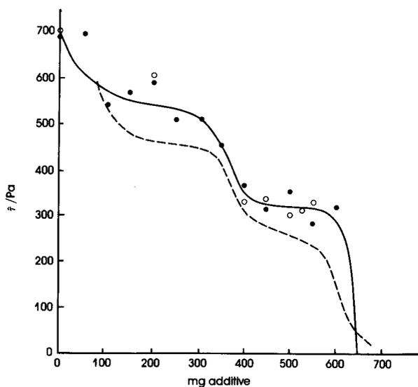
Fig. 6—Variation in flow stress barrier ( $\bar{\tau}$ ) of the  $\text{SiO}_2$ -5%  $\text{Fe}_2\text{O}_3$ - $\text{H}_2\text{O}$  slurry with increasing amounts of XP23/86 (— · — · —) and the titration curve of XP23/86 (— · — · —)
