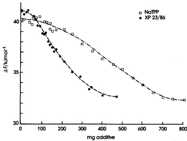
Fig. 4—Variation in flow activation energy ( $\Delta F$ ) of the WAGM slurry with increasing amounts of NaTPP (— · — · —) or XP23/86 (— · — · —)
