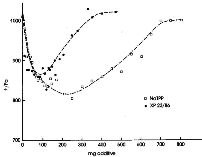
Fig. 7—Variation in flow stress barrier ( $\bar{\tau}$ ) of the WAGM slurry with increasing amounts of NaTPP (— · — · —) or XP23/86 (— · — · —)
