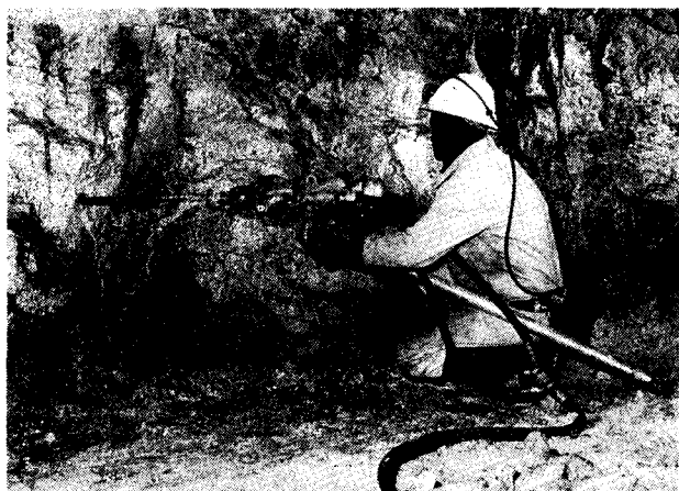
Fig. 3—Prototype water-powered rockdrill and thrustleg
