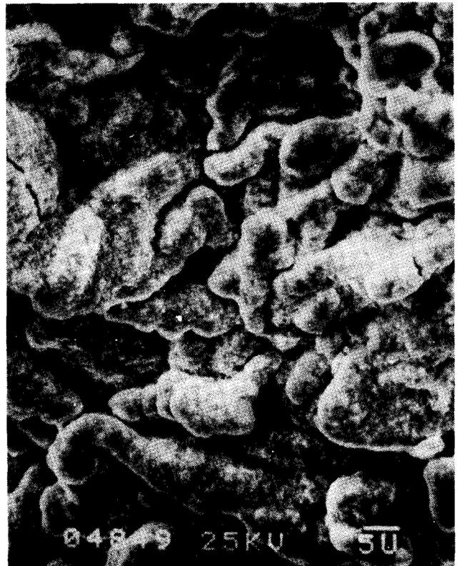
Fig. 9—Interdendritic morphology of a crack at the edge of a 'burnt' ingot of a duplex alloy (35 per cent chromium)
