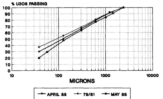
Fig. 8—Particle-size distribution of the uranium as a cumulative percentage of the total uranium
