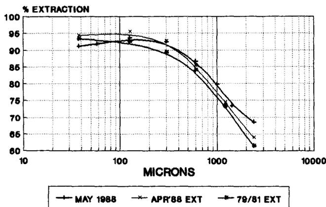
Fig. 9—Extraction efficiency at various particle sizes in 1979/1981, April 1988, and May 1988
