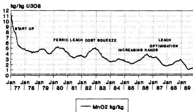
Fig. 4—Manganese consumptions from 1977 to 1988 (five-monthly moving averages) in kilograms per kilogram of  $U_3O_8$
