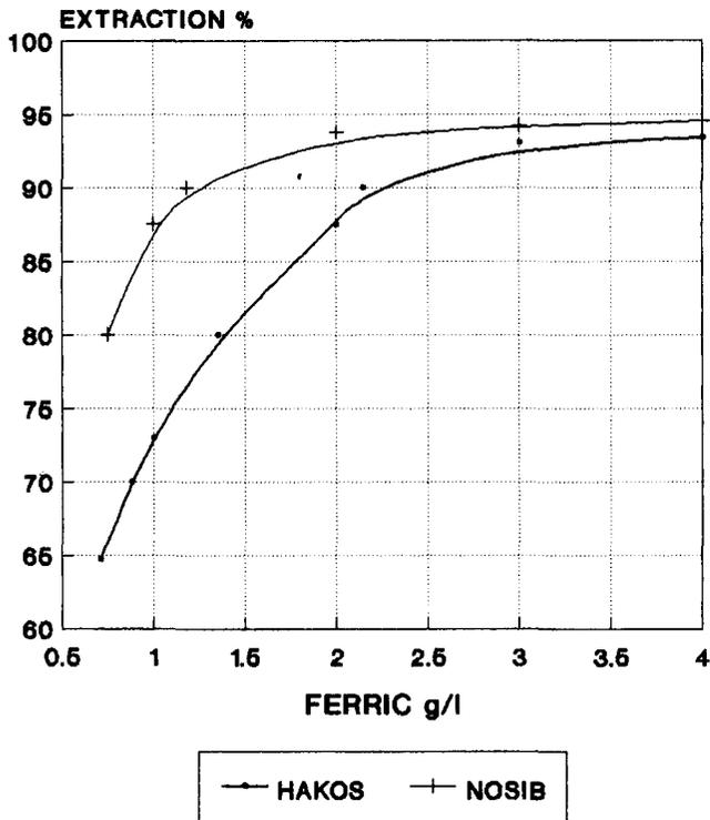
Fig. 1—The effect of Hakos and Nosib ores on the extraction (results obtained by Mintek)
