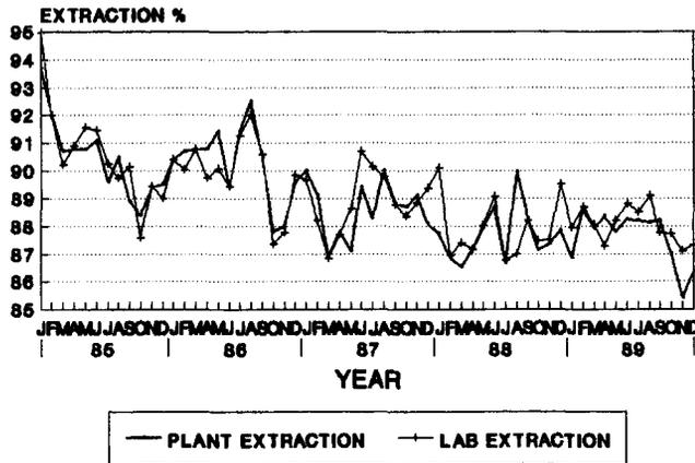
Fig. 5—Monthly extractions in the laboratory and on the plant
