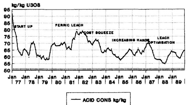
Fig. 3—Acid consumptions from 1976 to 1989 (five-monthly moving averages) in kilograms per kilogram of  $U_3O_8$
