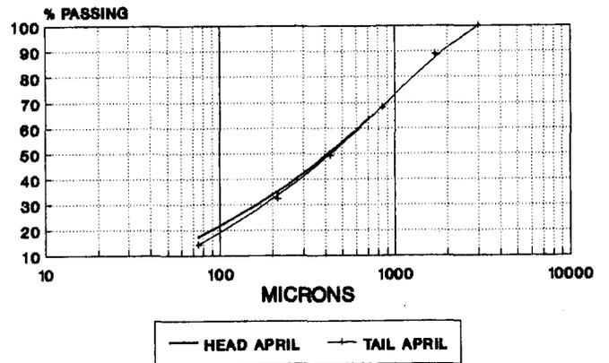
Fig. 7—Particle-size distribution in the head and in the tailings, April 1988
