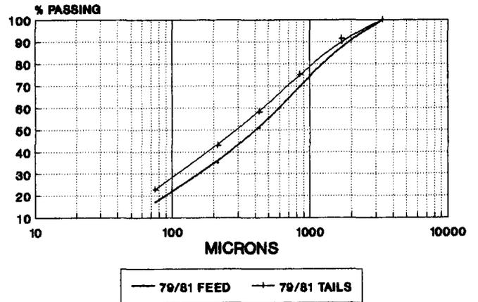
Fig. 6—Particle-size distribution in the feed to the leach and in the tailings, 1979 to 1981
