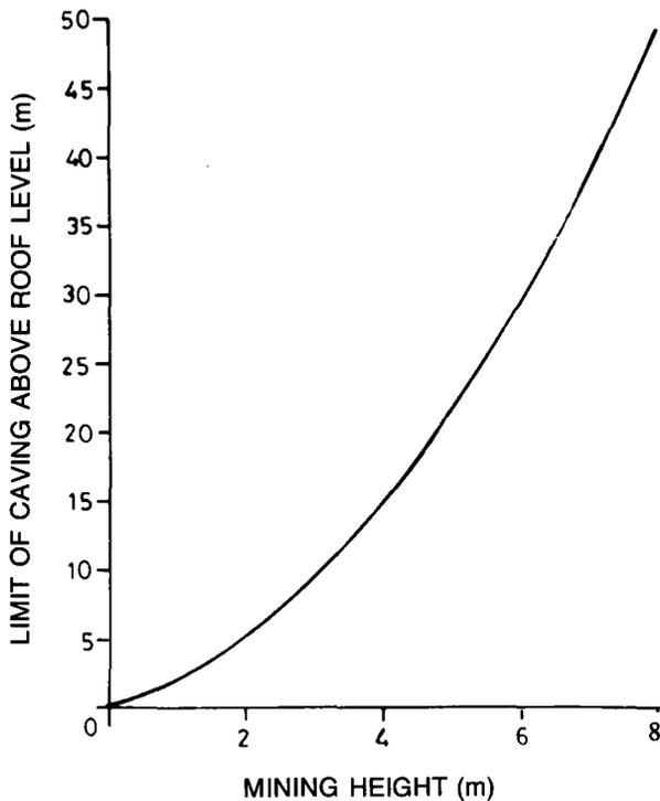
Fig. 3—Extent of caving above roof level for different thicknesses of extracted seam
