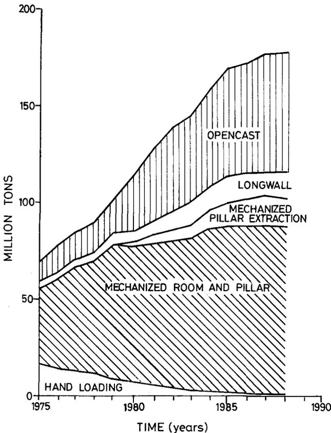
Fig. 2—Mining method used for the production of coal in South Africa
