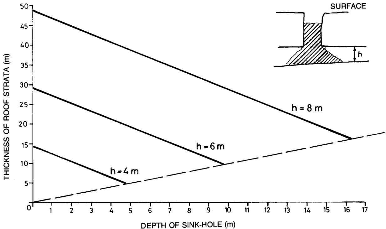
Fig. 4—Depths of sink-hole for different extraction heights
