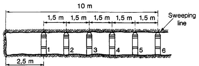
Fig. 1—Section of a stope showing the first six lines of profile props
