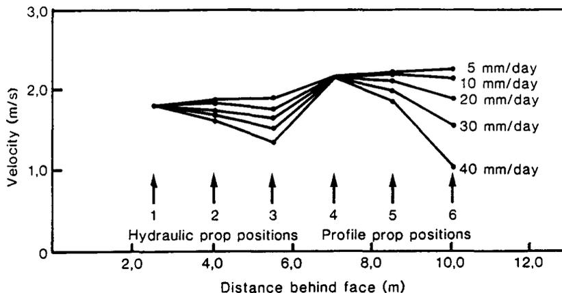
It is of interest to note that, where yielding timber support systems are used and stope-closure rates of 10 mm to 20 mm per day occur, there is effectively no back-area support further than 10 to 20 m behind the stope face, all the units having failed at that distance. It is estimated that 10 to 15 per cent of the industry is mining with no effective back-area support except gully packs.
