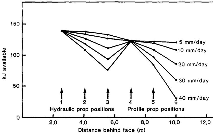
Fig. 7—Measure of the ability of a support system to absorb energy as a function of the distance behind the stope face for various closure rates
