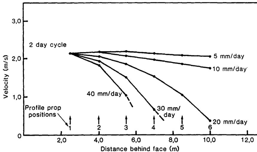
Fig. 8—Minimum ground velocity that will cause profile props to fail for different distances behind the slope face at various closure rates
