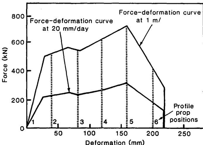
Fig. 3—Positions of profile props in relation to the force-deformation curve for a closure rate of 20 mm per day
