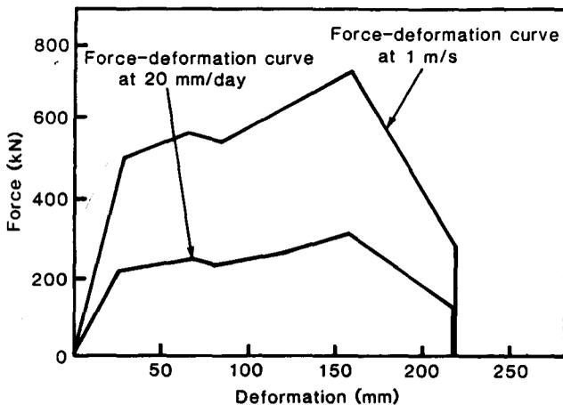
Fig. 2—Force-deformation curves for a profile prop at various deformation rates
