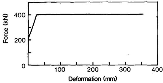
Fig. 6—Force–deformation curve for a 400 kN hydraulic prop
