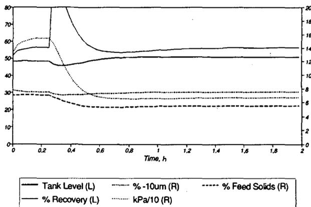
Fig. 12—Typical dynamic responses obtained from the single-variable model:
