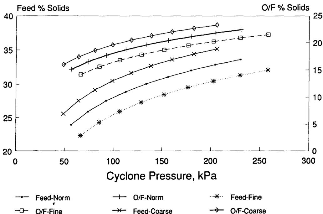
Fig. 10—Solids content versus hydrocyclone pressure
