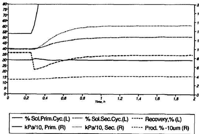
**Fig. 8—Dynamic response obtained from the two-stage system without recycle:**
