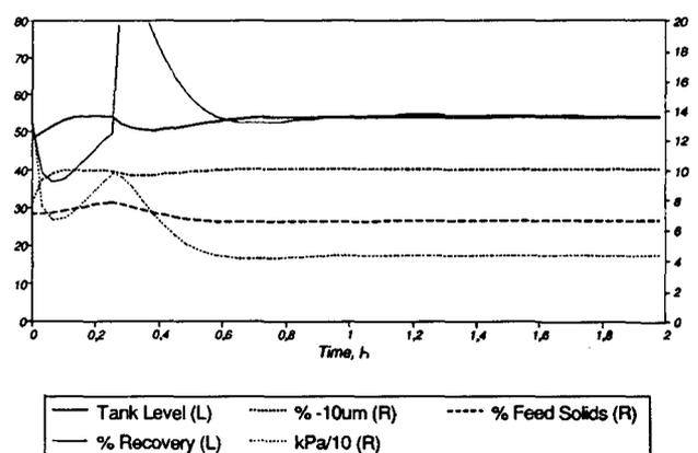
Fig. 13—Typical dynamic responses obtained from the two-variable model:
