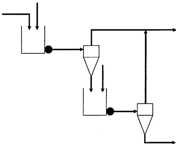
Fig. 2—The two-stage circuit without recycle
