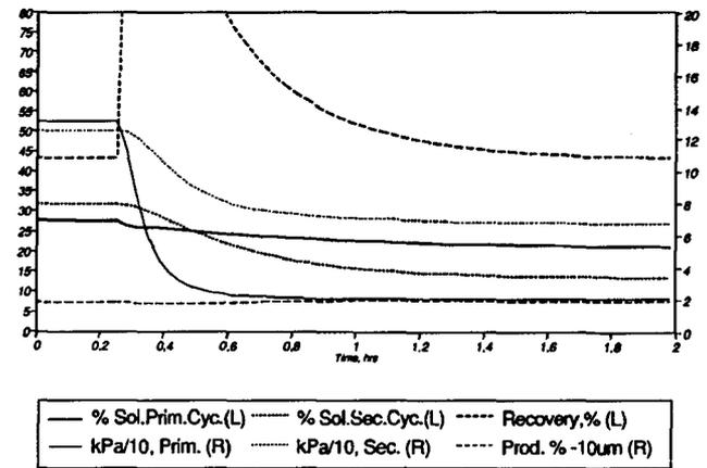
**Fig. 9—Dynamic response obtained from the two-stage system with recycle:**
