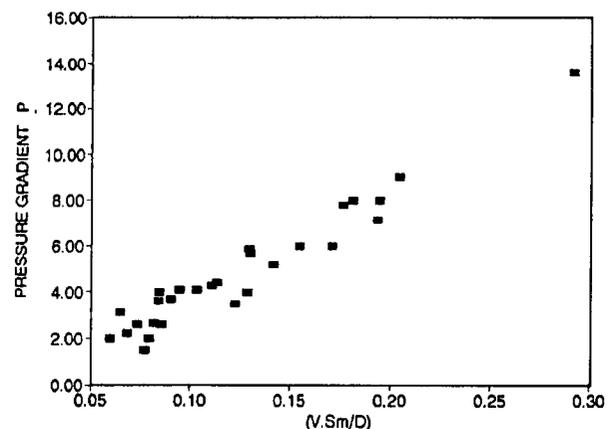
Fig. 8 - Pressure gradient versus transportation parameters
