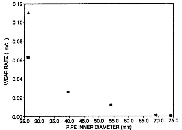
Fig. 6a—Pipe inner diameter versus rate of pipe wear
