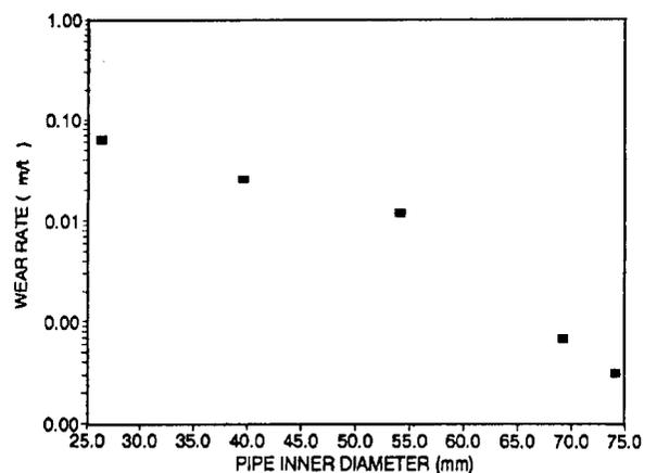
Fig. 6b—Pipe inner diameter versus log rate of pipe wear
