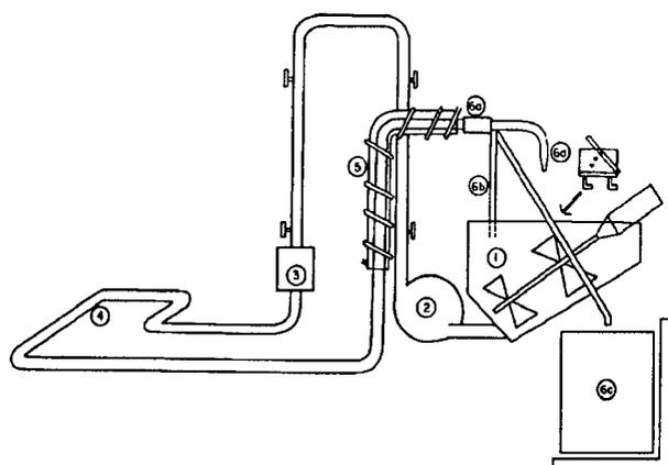
Fig. 1 – The closed-loop test pipeline
