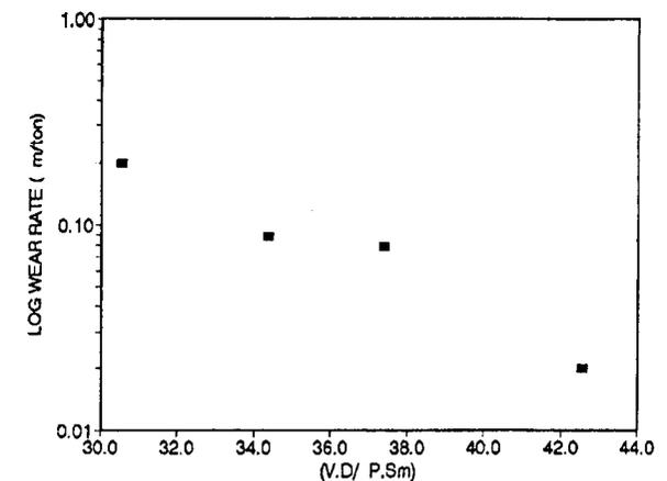
Fig. 7—Transportation parameters versus rate of wear
