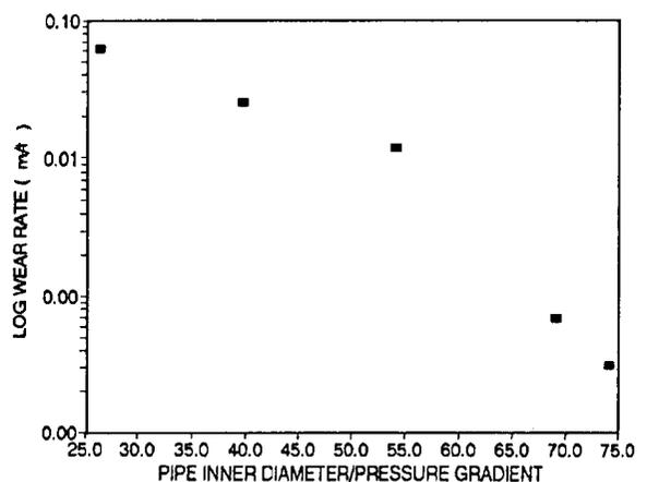
Fig. 6c – Pipe inner diameter/pressure gradient versus rate of pipe wear (3,0 m/s)
