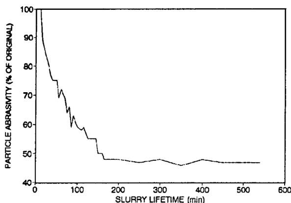
**Fig. 3**—Particle degradation as a percentage of particle abrasivity
