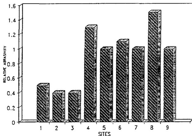
Fig. 9—Backfill sites versus relative abrasivity
