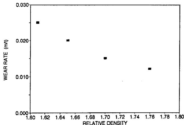
**Fig. 4**—Relative density of slurry versus rate of pipe wear
