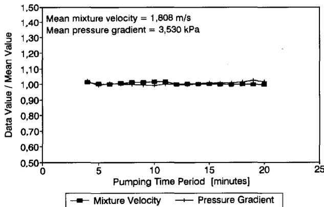
Figure 3—Variation of mixture velocity and pressure gradient with time for a slurry containing 5.1 per cent binder and having a relative density of 1,69
