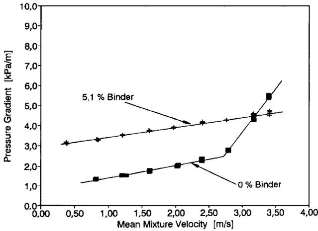
Figure 6—Variation of mixture velocity and pressure gradient for slurries with and without binder at a relative density of 1,69
