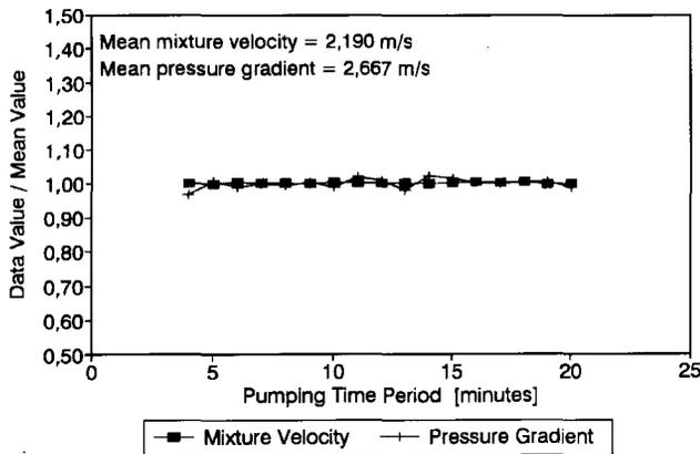
Figure 2—Variation of mixture velocity and pressure gradient with time for a slurry containing 5.4 per cent binder and having a relative density of 1,65
