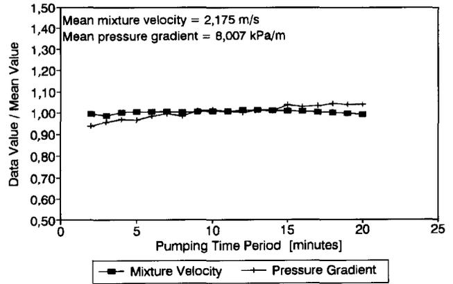
Figure 4—Variation of mixture velocity and pressure gradient with time for a slurry containing 4.8 per cent binder and having a relative density of 1,72
