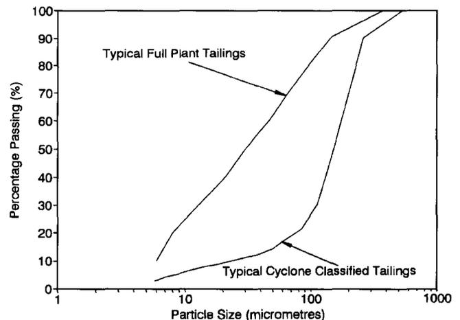
Figure 1—Particle-size distribution in two tailings slurries
