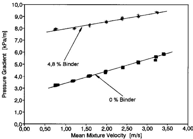
Figure 7—Variation of mixture velocity and pressure gradient for slurries with and without binder at a relative density of 1,72
