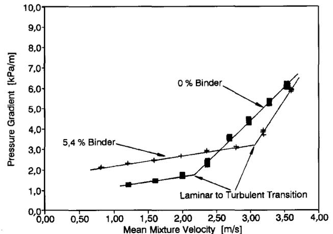
Figure 5—Variation of mixture velocity and pressure gradient for slurries with and without binder at a relative density of 1,65
