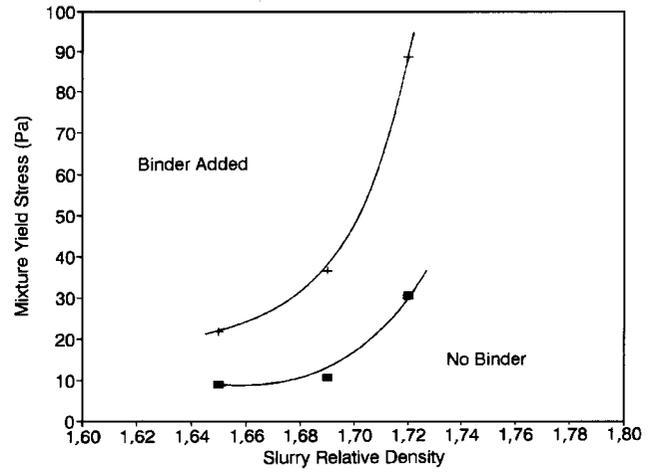
Figure 8—Variation in yield stress and relative density for slurries with and without binder
