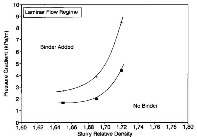
Figure 9—Variation in pressure gradient with relative density for slurries with and without binder at a mean velocity of 2,0 m/s
