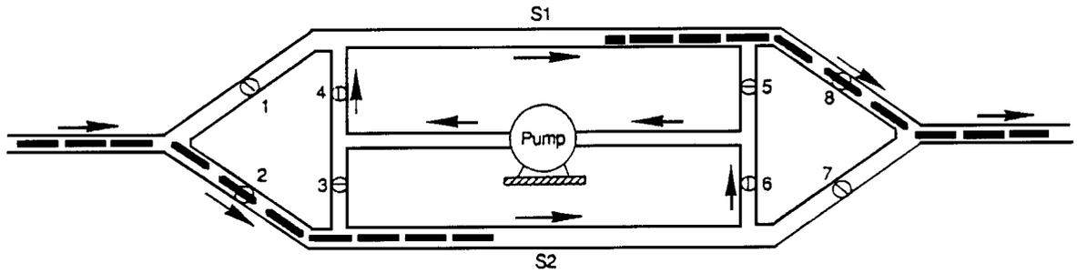
S1 = Line 1, S2 = Line 2, 1 to 8 = Computer-controlled valves, — = Coal logs
