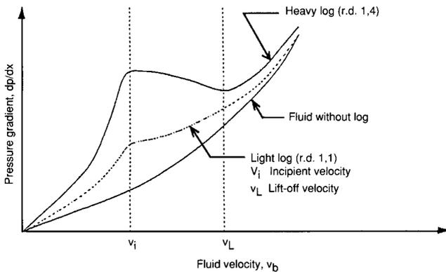
Figure 4—Variation of pressure gradient with velocity in a horizontal pipe. (After Paksanonda<sup>5</sup>)
