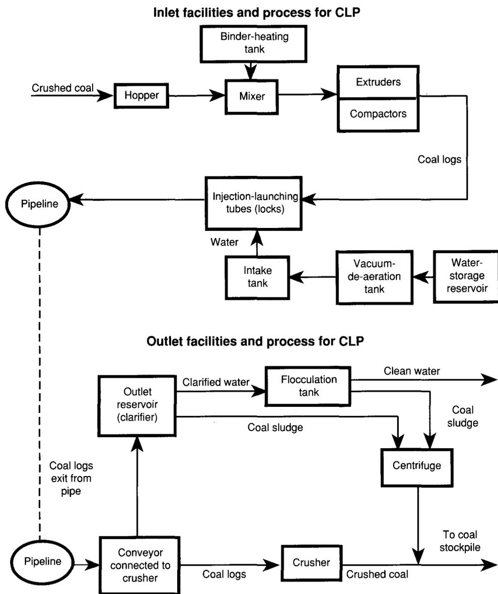
**Figure 1—Conceptual flowchart of coal-log-pipeline system**
