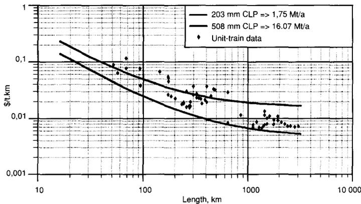
**Figure 2—Unit-cost and unit-distance cost for transportation of coal unit train and CLP**
