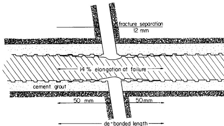
Figure 2—Section through a fully grouted re-bar, showing necking and start of fracture after limited opening of the separation surface
