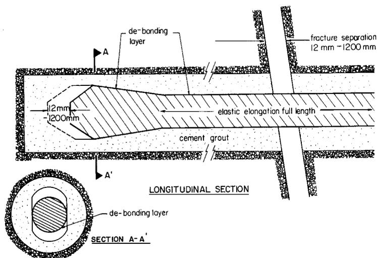
Figure 3—Section through a cone bolt, showing its ability to yield limited only by the length of the hole beyond the separation surface
