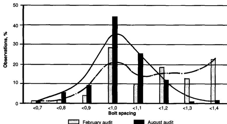
Figure 4—Distribution of distances (actual measurements) between bolts with a pattern of 1,0 m designed spacing (after Wilkes<sup>7</sup>)
