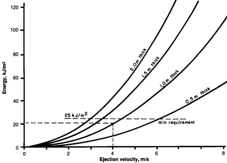
Figure 5—Kinetic energy as a function of ejection velocity for rock slabs of various thicknesses
