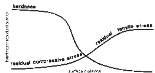
Figure 1—Hardness and residual stress in a laser-treated skin (schematically)
