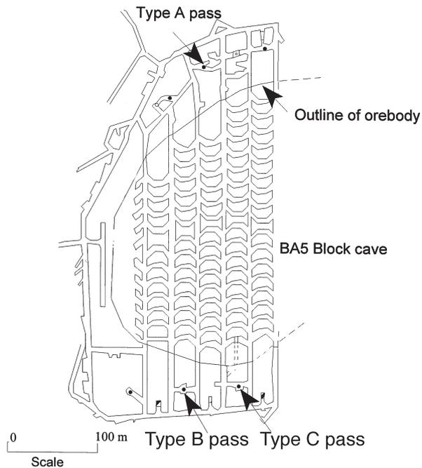
Figure 1—Plan showing layout of BA5 Block Cave and position of passes
