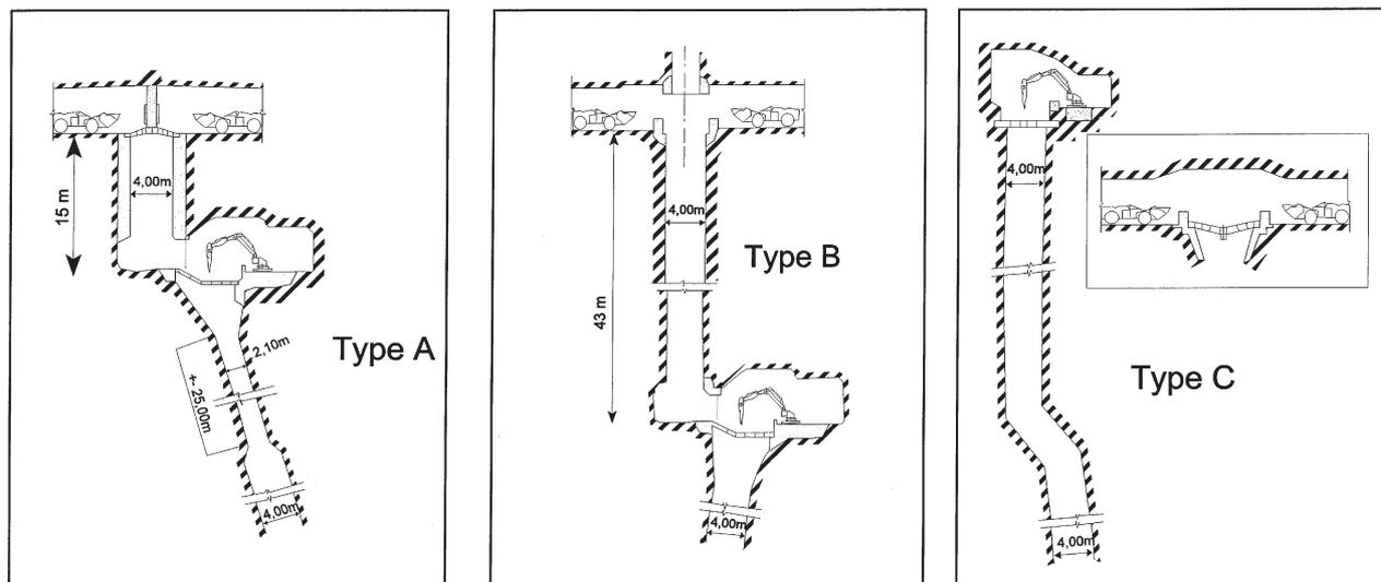
Figure 3—Three rock breaker layouts evaluated
