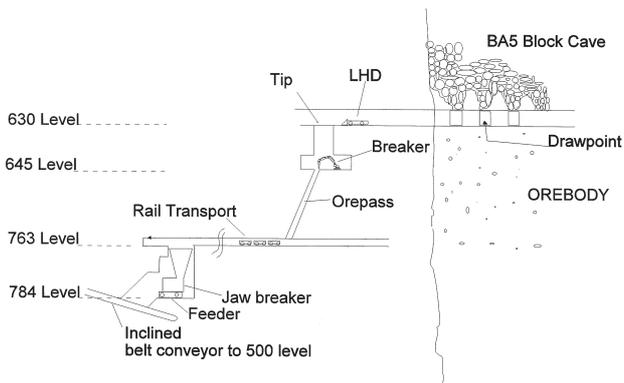
Figure 2—Schematic section showing flow of ore from drawpoints to inclined conveyor
