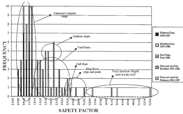
Figure 1—Frequency of pillar collapse versus design safety factor
