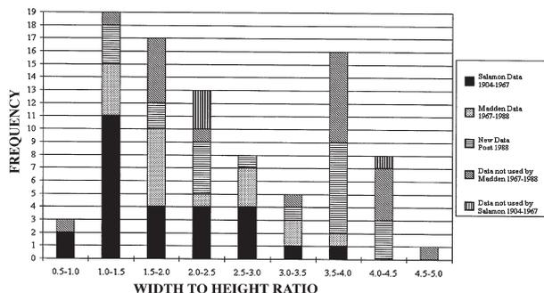
Figure 2—Frequency of pillar collapse versus width to-height ratio
