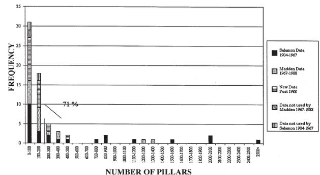
Figure 3—Frequency versus number of collapsed pillars
