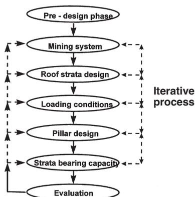
Figure 6—Conceptual pillar system design methodology
