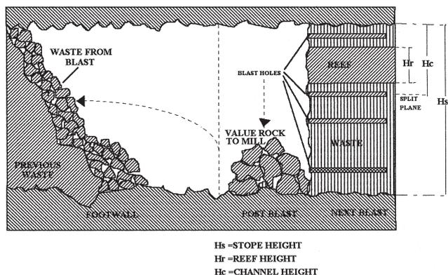
Figure 1—Selective blast mining. Section through stope
