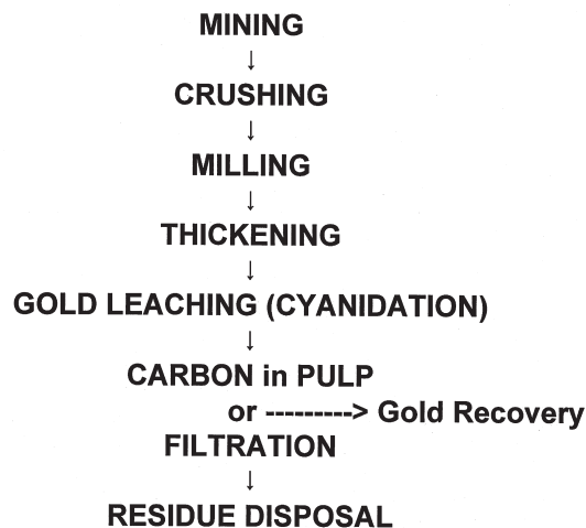
Figure 1—The simplest gold recovery process. Very low potential for radiation hazard from fortuitous gravity concentration (for example in launders)
