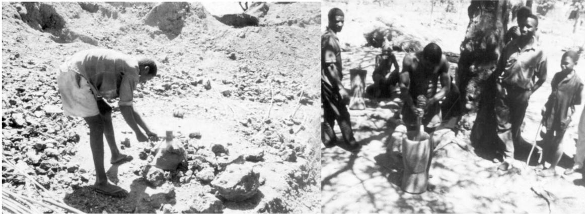
Figure 1—Basic comminution technique, using hammer and pounder
