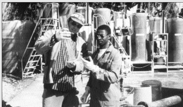
Evaluation of the SAVMIN process for treating acid mine drainage at Grootvlei Gold Mine
