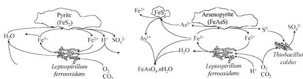
Figure 1—Diagrammatic representation of the bioleaching of pyrite and arsenopyrite via the two-step mechanism. The bacteria shown are planktonic (i.e., unattached) for reasons of clarity; however, the mechanism is the same for both attached and unattached micro-organisms (after Breed *et al.*<sup>19</sup>)
