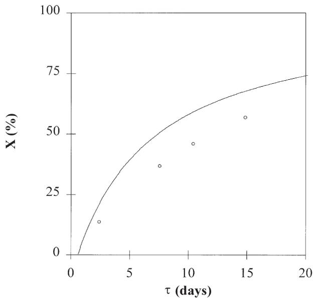
Figure 7—Comparison between the predicted variation in the pyrite conversion with changing residence time for a [—] *Leptospirillum*-like bacterium and the [O] experimental results obtained by Hansford and Chapman<sup>6</sup>. Data were calculated from the results of Van Scherpenzeel *et al.*<sup>68</sup> (after Breed<sup>19</sup>)
