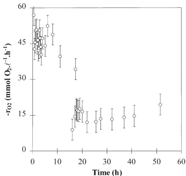
Figure 4—Variation in the oxygen utilization rate during the disruption test carried out using the primary bioreactor. The error bars represent the measured  $-r_{O_2} \pm$  the average variation in  $-r_{O_2}$  measured during steady-state operation, at  $\tau=4$  days (after Breed *et al.*<sup>25</sup>)
