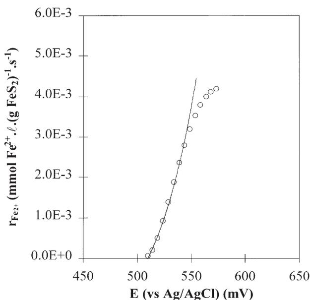
Figure 5—Comparison between the [—] Butler-Volmer based model prediction ( $r_0 = 5 \times 10^4$ ,  $\alpha = 0.498$ ,  $\beta = 0.0272$ ,  $E' = 510$ ) and the [O] experimental leaching rate data (after Ruitenberg *et al.*<sup>54</sup>).
