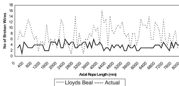
Figure 5—Lloyds Beal: Broken wire comparison for Test 3 at 100 mm intervals
