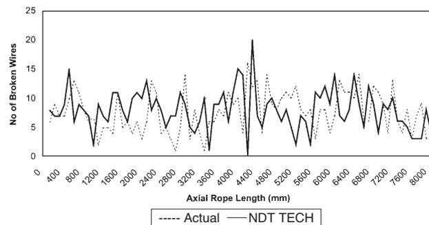
Figure 6—NDT Technologies: Broken wire comparison for Test 2 at 100 mm intervals
