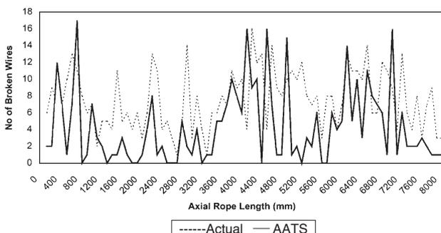
Figure 8—AATS: Broken wire comparison for Test 2 at 100 mm intervals
