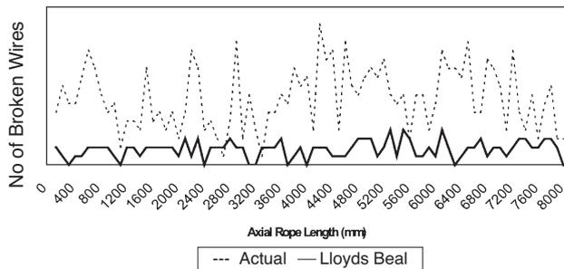
Figure 4—Lloyds Beal: Broken wire comparison for Test 2 at 100 mm intervals
