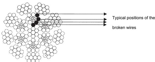
Figure 1—Position of broken wires within a multi-layer, low rotation rope sample
