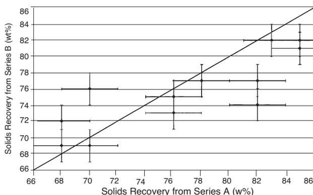
Figure 5—Comparison of solids recoveries from duplicate runs
