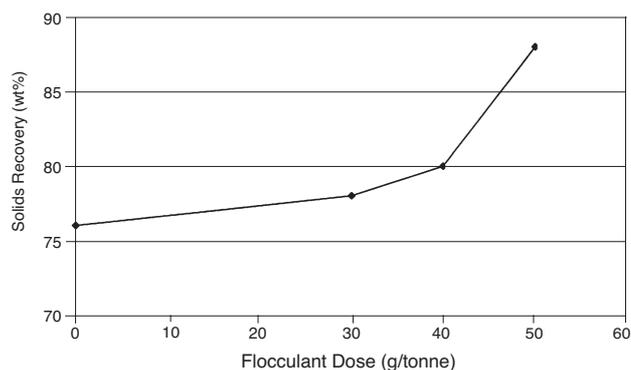
Figure 11—Effect of flocculant dose on solids recovery
