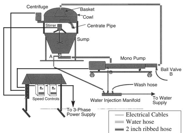
Figure 3—Pilot-scale fine coal centrifuge circuit
