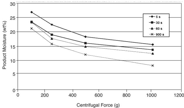
Figure 2—Effect of centrifugal force on product moisture
