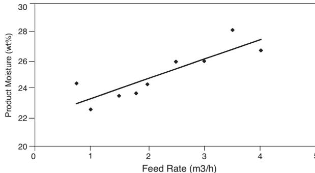
Figure 8—Effect of feed rate on product moisture
