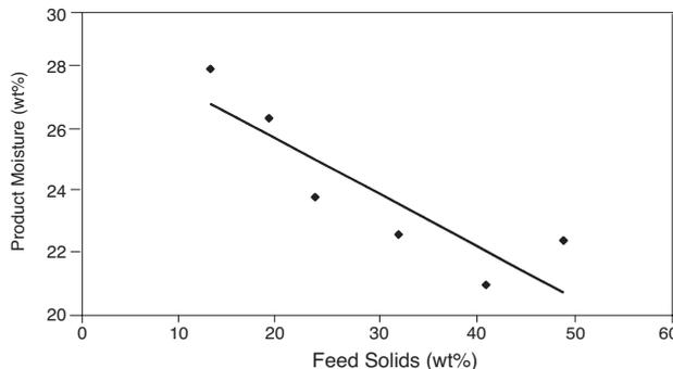
Figure 9—Effect of feed solids on product moisture
