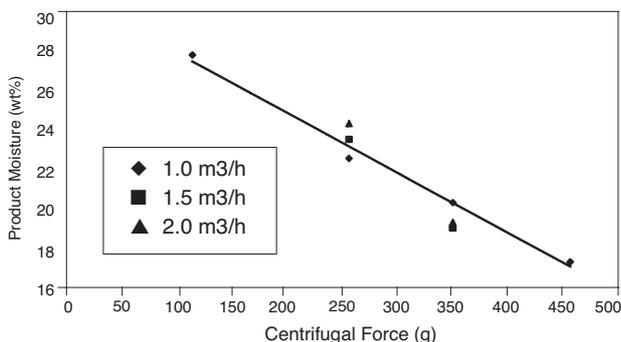
Figure 7—Effect of centrifugal force on product moisture
