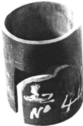
Figure 10—'Bursting' pipe failure at air-backfill interface
