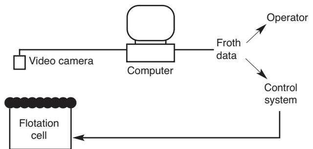
Figure 9—Schematic of the froth image analysis system
