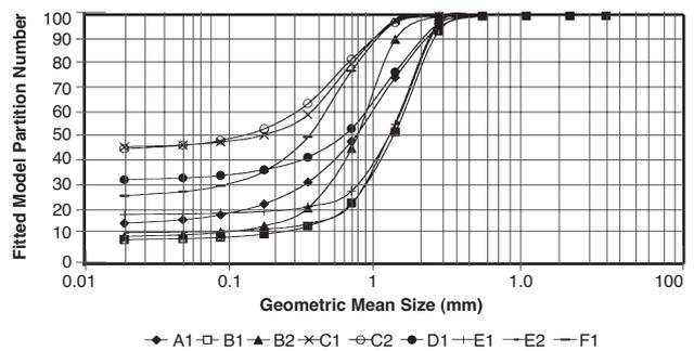
Figure 3—All modified Whiten model fitted drain section data (B2 sieve bend/low head with 0.55 mm aperture; C1, C2, F1 banana screens with aperture 0.56 to 0.8 mm; the rest banana screens with apertures 1.1 to 1.7 mm)
