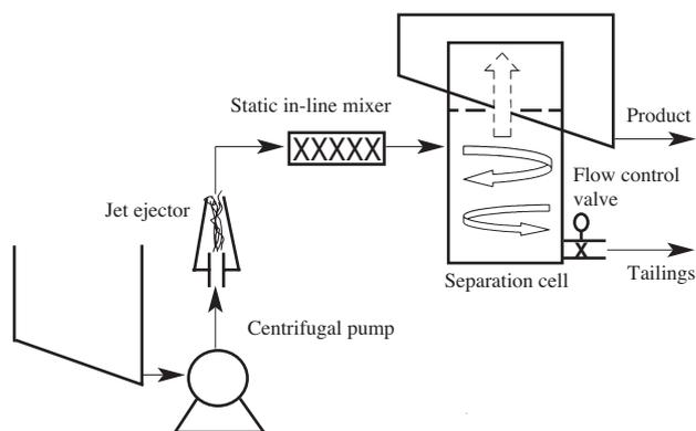
Figure 7—The TurboFlotation system
