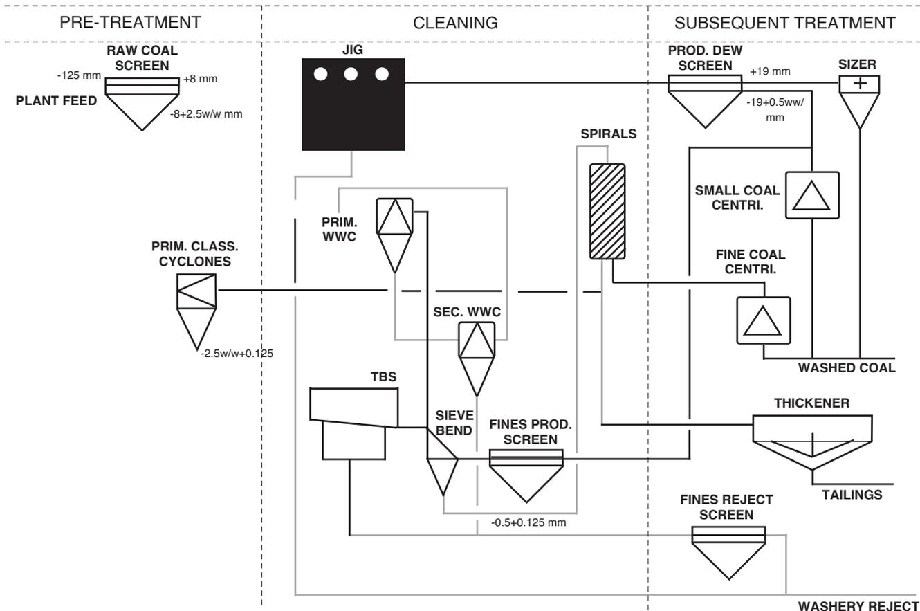
Figure 6—Bayswater TBS™ plant upgrade as-built process flowsheet
