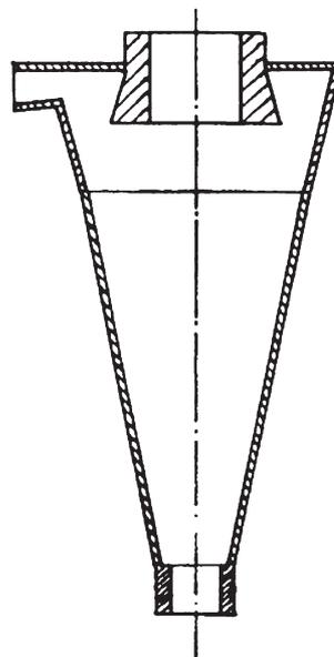
Figure 5—Schematic drawing of the new cyclone design concept from JKMRC
