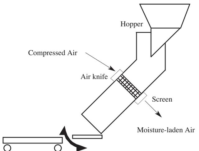
Figure 10—Schematic of the pilot scale jet chute
