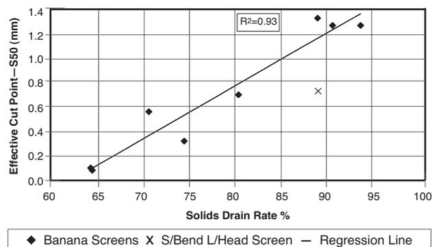
Figure 4—Solids drain rate% v effective cut point (S50) with sieve bend/low head data point shown
