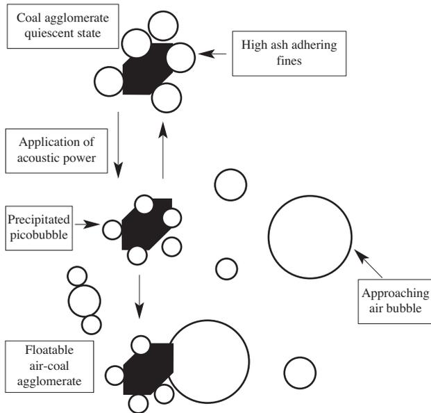
Figure 8—A proposed mechanism for picobubble assisted flotation
