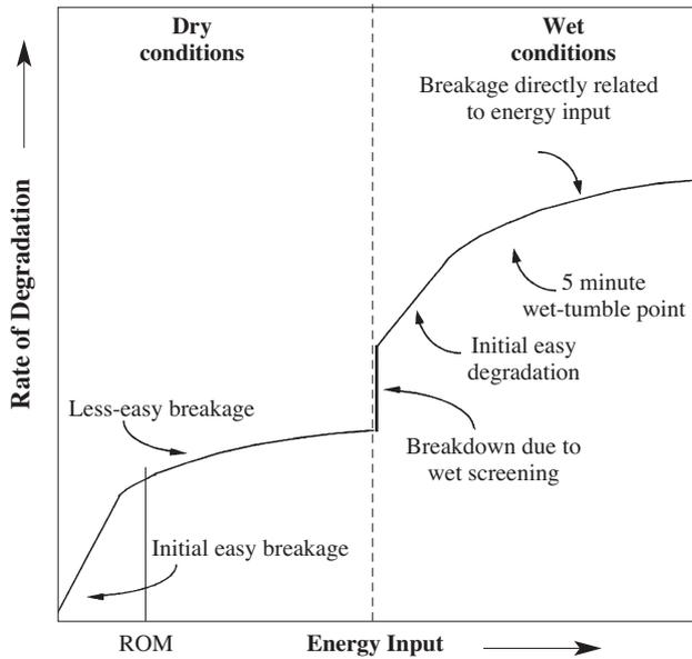
Figure 1—Conceptual breakage model for coal handling and preparation
