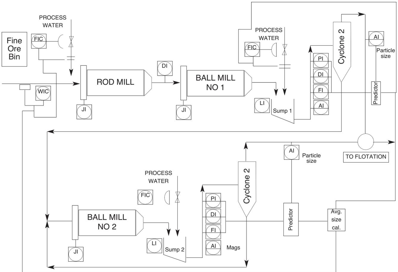
Figure 1—Schematic of milling circuit
