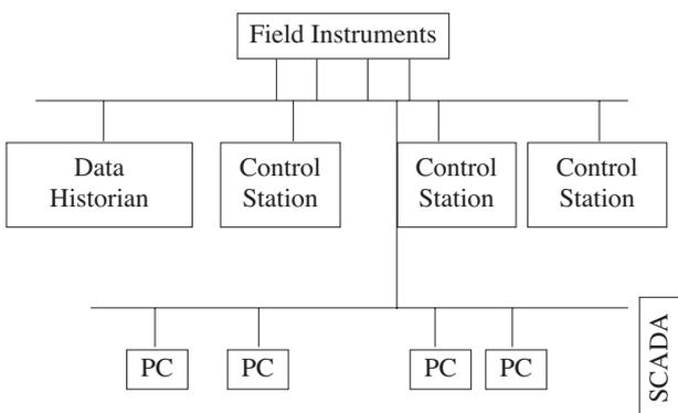
Figure 2—Schematic of the control system
