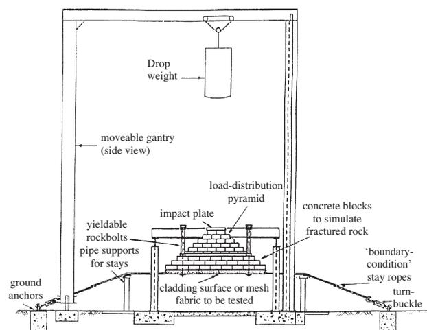
Figure 2—Dynamic test loading facility
