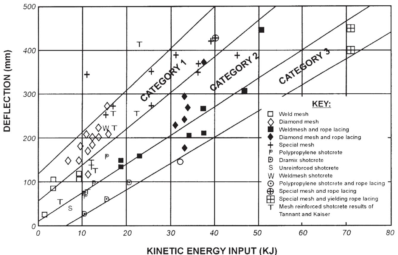
Figure 3—Results of dynamic testing of membranes
