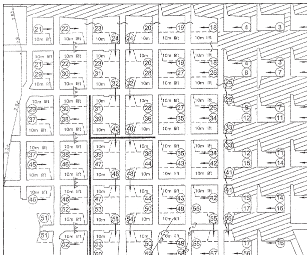
Figure 11—Partial pillar extraction sequence at Colliery G
