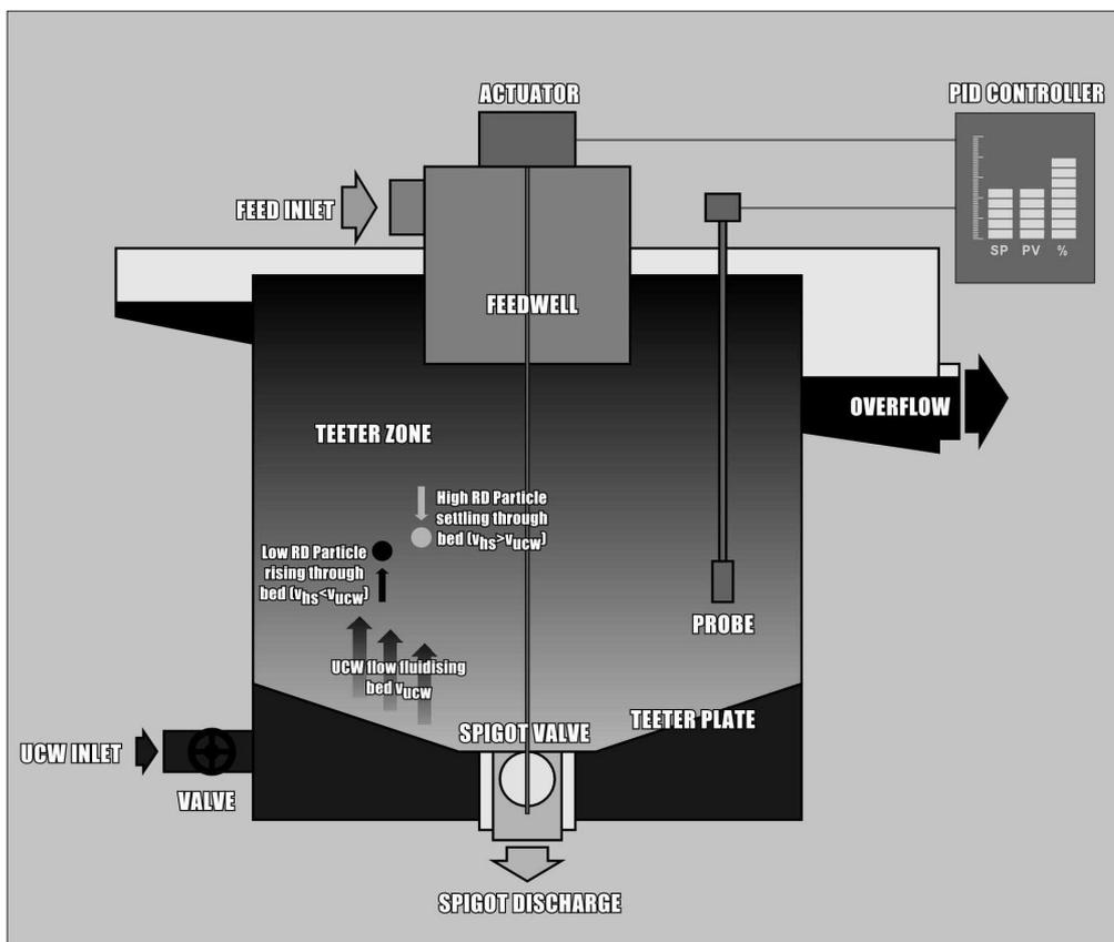
Figure1—TBS machine—principles of operation
