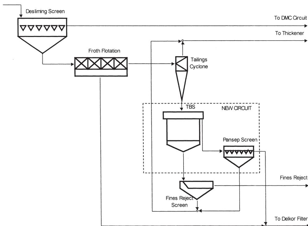
Figure 6—Goonyella/Riverside No. 1 CPP froth flotation circuit upgrade
