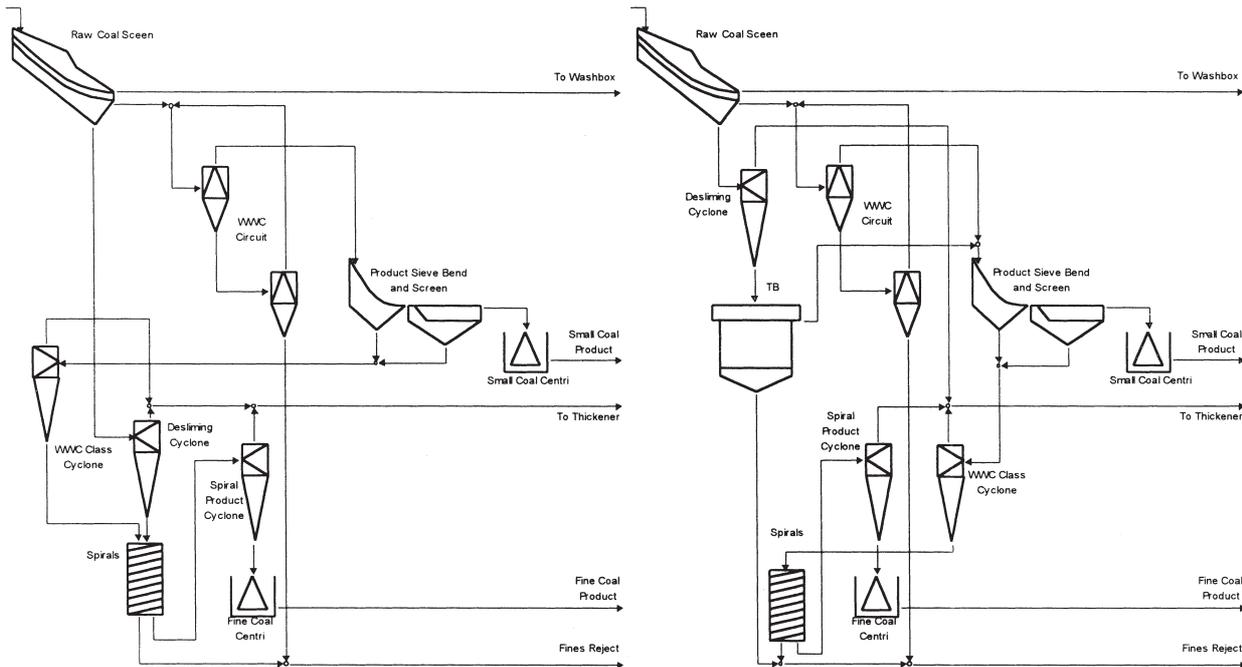
Figures 4 and 5—Bayswater fine coal circuit flowsheets before and after TBS upgrade
