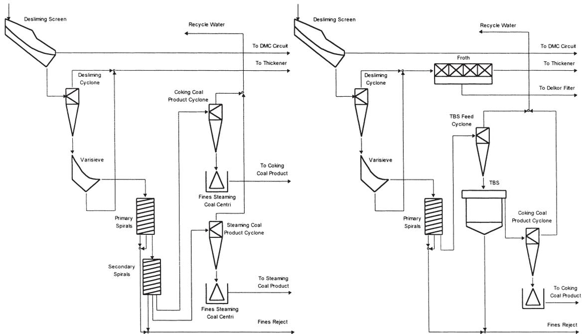
Figures 2 and 3—Stratford fine coal circuit flowsheets before and after flotation circuit upgrade
